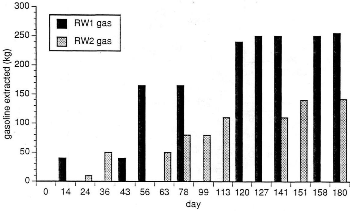
Fig. 4. Cumulative mass of gasoline extracted by RW1 and RW2 following the indicated time of VES operation.
