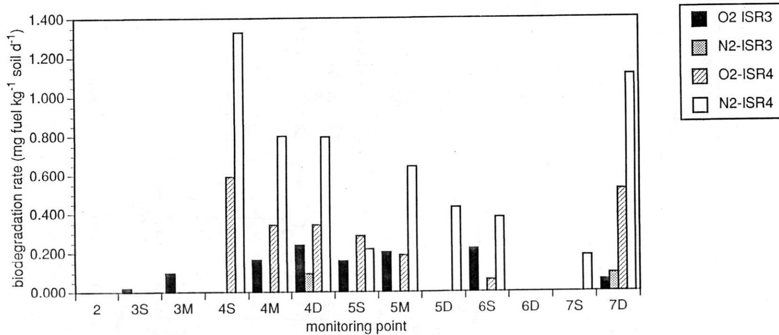
Fig. 9. Estimated aerobic(O<sub>2</sub>) and anaerobic (N<sub>2</sub>) biodegradation rates in ISR tests 3 and 4.
