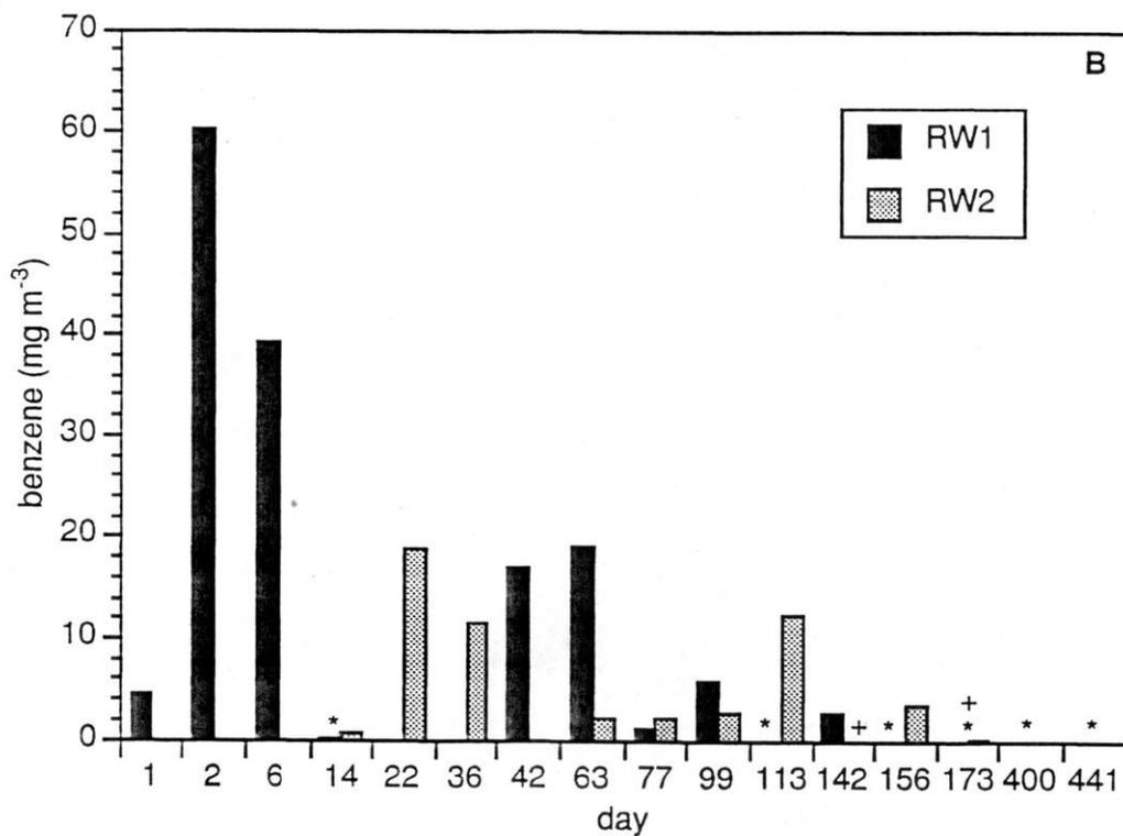
Fig. 2. Gasoline (A) and benzene (B) vapor concentrations in extraction well off-gases. In A, low level gasoline detections at RW1 (\*) were (day); 0.7 (14), 4 (113), 0.5 (156), 1.5 (173), 6 (400), 0 (410). Low level gasoline detection at RW2 (+) was 1.0 (173). In B, low level benzene detections at RW1 (\*) were (day); 0.04 (14), 0 (113), 0 (156), 0.03 (173), 0 (400) and 0 (410). Low level benzene detections at RW2 (+) were (day); 0 (142), 0.03 (173).
