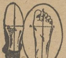
**STRAIGHT**—where the surface across the ball (A-B) is equal on either side of the line (C-D).
