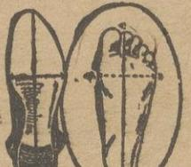
**OUTFLARE**—where more of the surface across the ball (A-B) is outside the line instead of inside the line (C-D).
