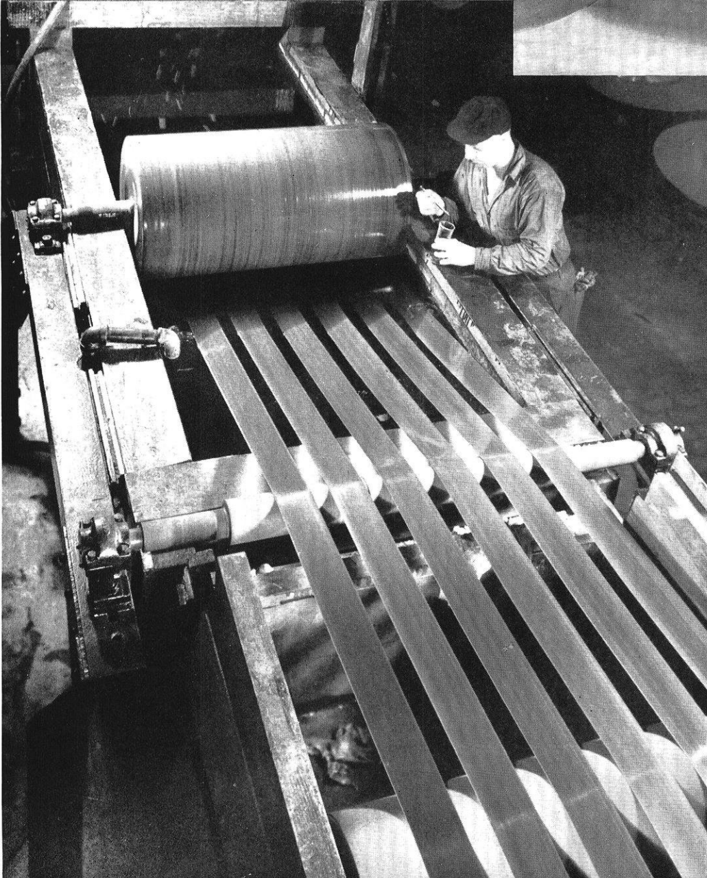
Fig. 16. (Left), Continuous pickling of cold-rolled stainless strip after annealing, Cuyahoga Works.
