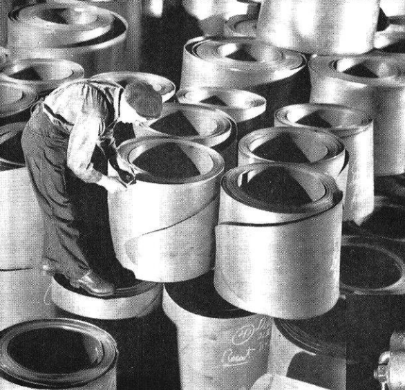
Fig. 4. (At left). Coils of hot-rolled stainless strip which will be further processed into cold-rolled strip or will be cut into breakdowns for rolling into sheets. The employee is putting a micrometer on the edges to see whether they are of the right thickness. This is called "inspecting for accuracy of gage." Gary Works, Carnegie-Illinois Steel Corpn., Gary, Ind.
