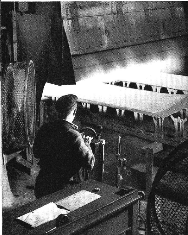
Fig. 7. (Below). Continuous annealing furnace, Wood Works, Carnegie-Illinois, in which stainless steel sheets are heat treated. The stainless sheet is laid on a "rider" or "waster" sheet for its ride through the furnace. The conveying mechanism is below the furnace except for the dogs (supports projecting from a continuous chain belt) which hold the sheets. The dogs project through slots in the furnace bottom. Note the two ventilating fans which help to keep the operator comfortable.
