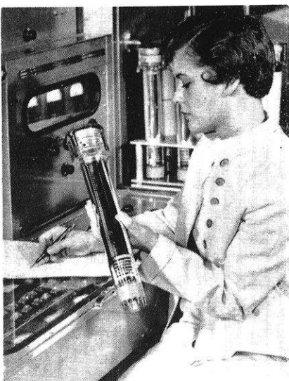
The "Cat Eye", as announced recently by the Air Force, is approximately a thousand times more sensitive than the standard television camera, and permits pilots to "see in the dark with daylight clarity."
