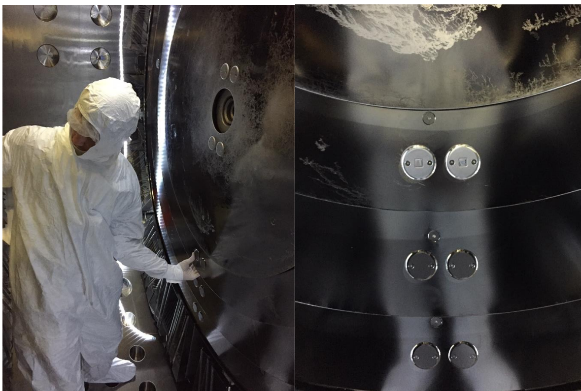
Figure 3-11. Installment of graphene coated and uncoated samples in C-2W. Courtesy of TAE Technologies team.
