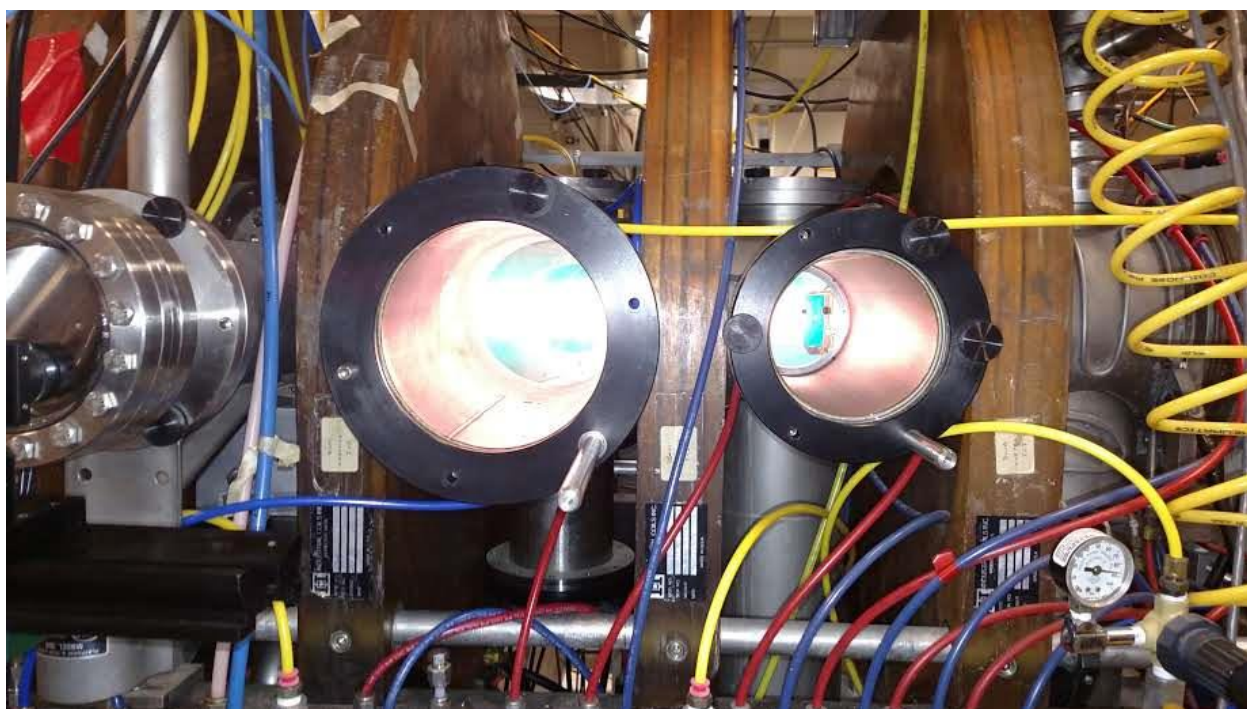
Figure 3-7. Deuterium plasma exposure to tungsten disks in PISCES-A for 30 minutes.
