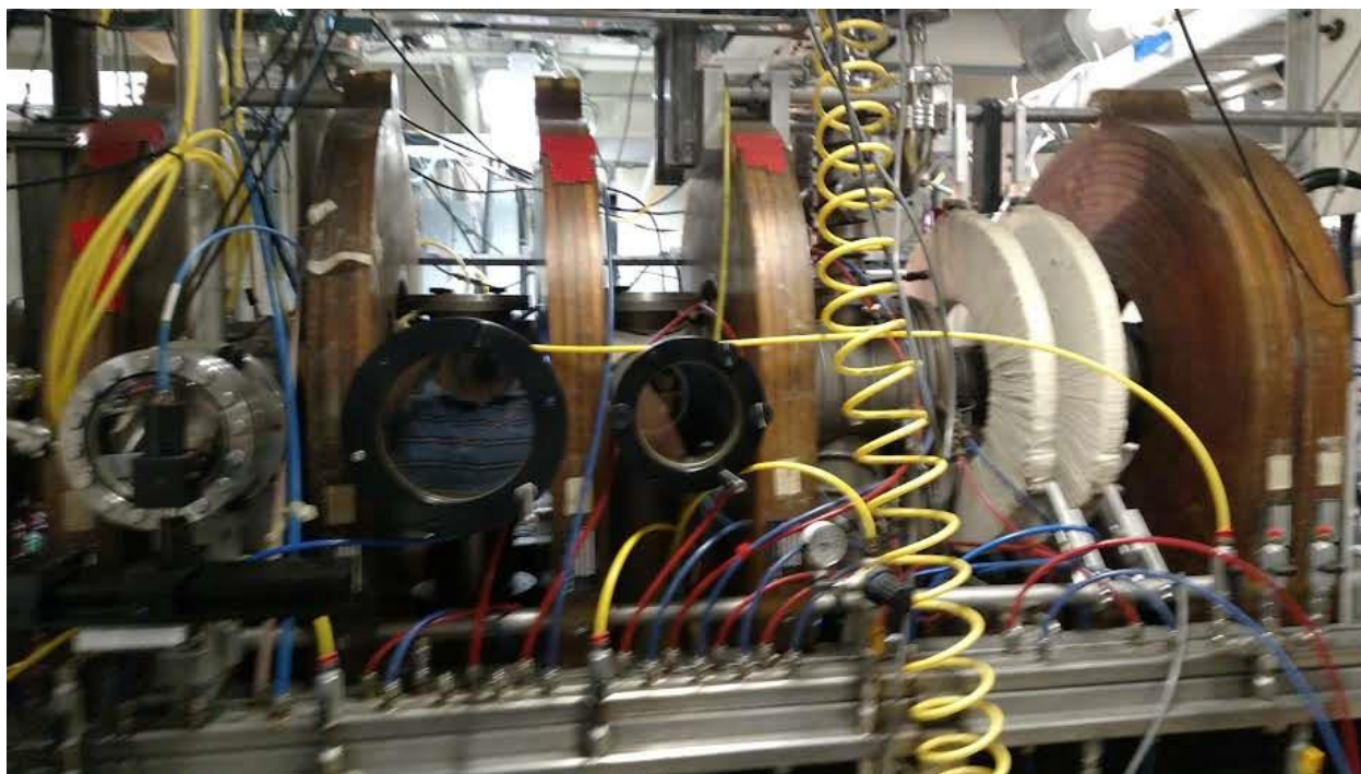
Figure 3-6. PISCES-A vacuum chamber and magnetic coils at the University of California-San Diego.
