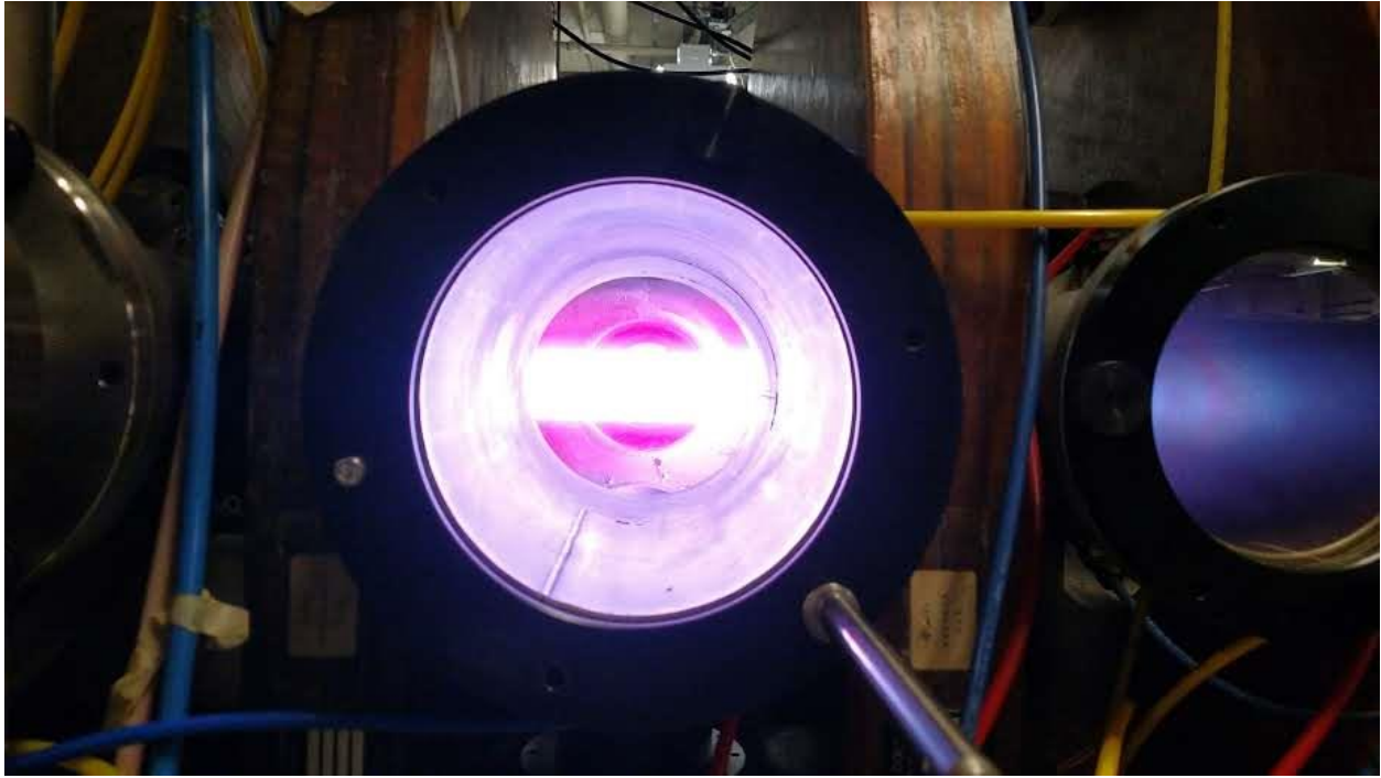
Figure 3-8. Helium plasma exposure to tungsten disks in PISCES-A for 30 minutes.
