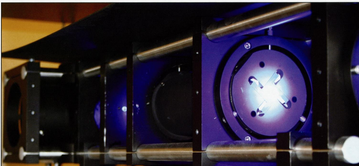
Located in the NanoTech Lab, the microarray synthesizer is an essential instrumentation device for researching the specific genes of diatoms.
