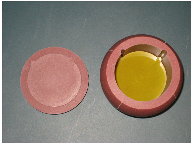
Figure 4.2: The film stack dosimeter phantom, which maintains the radial alignment of the films.
