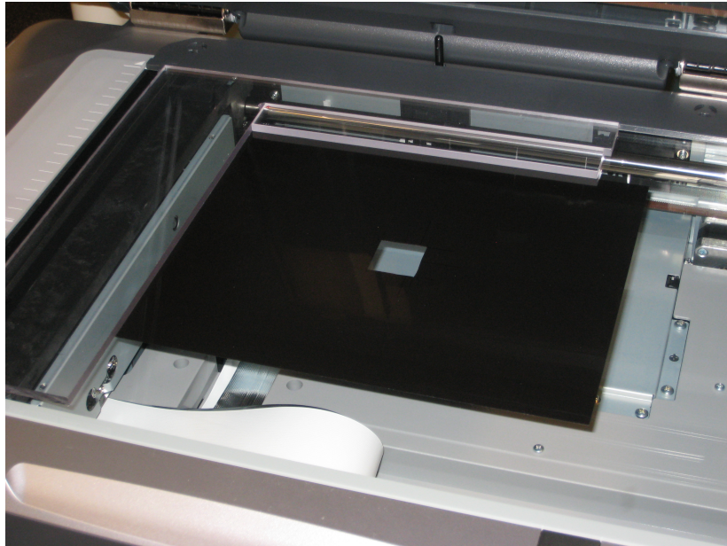
Figure 3.2: Image of the flatbed document scanner used to read films. The polycarbonate frame used for positioning reproducibility and the film masks are shown on the scanbed.
