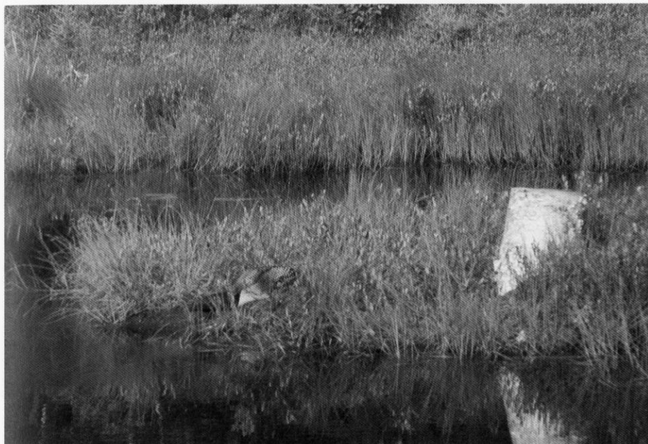
Figure 2. Camera monitoring an artificial Common Loon nest. The camera is inside a housing camouflaged with birch bark.
