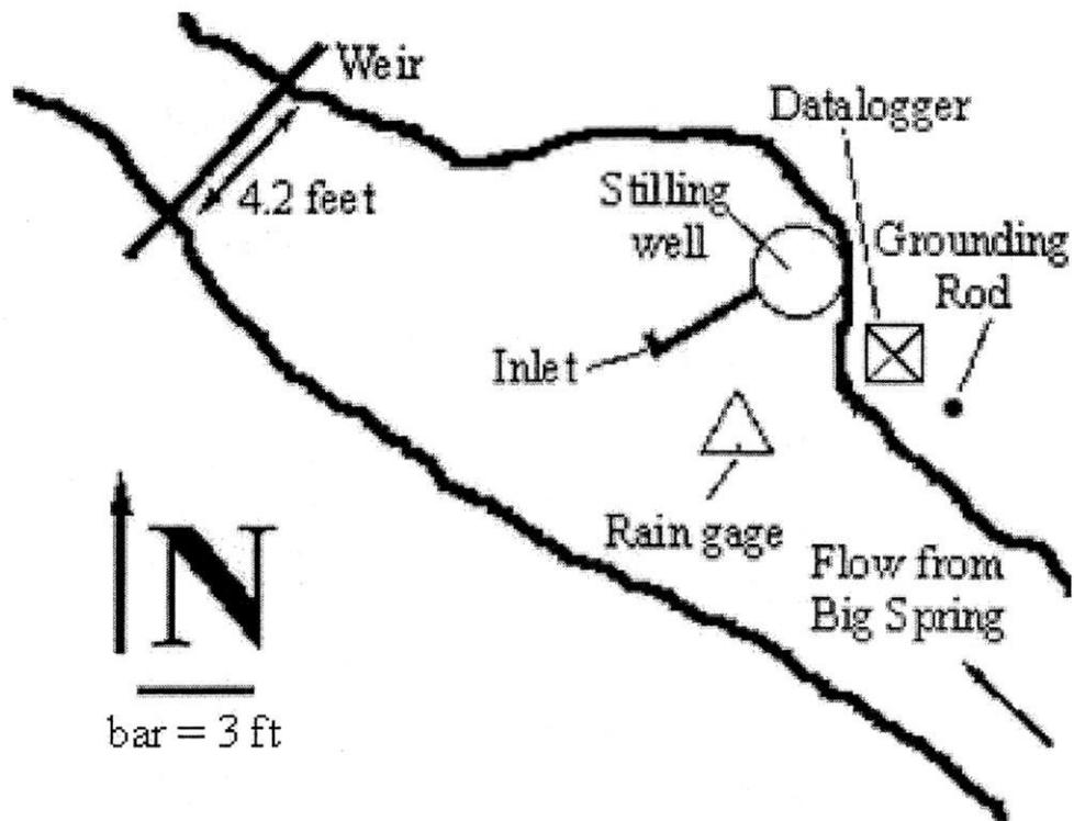
Figure 35. Layout of Gunflint Trail weir monitoring equipment
