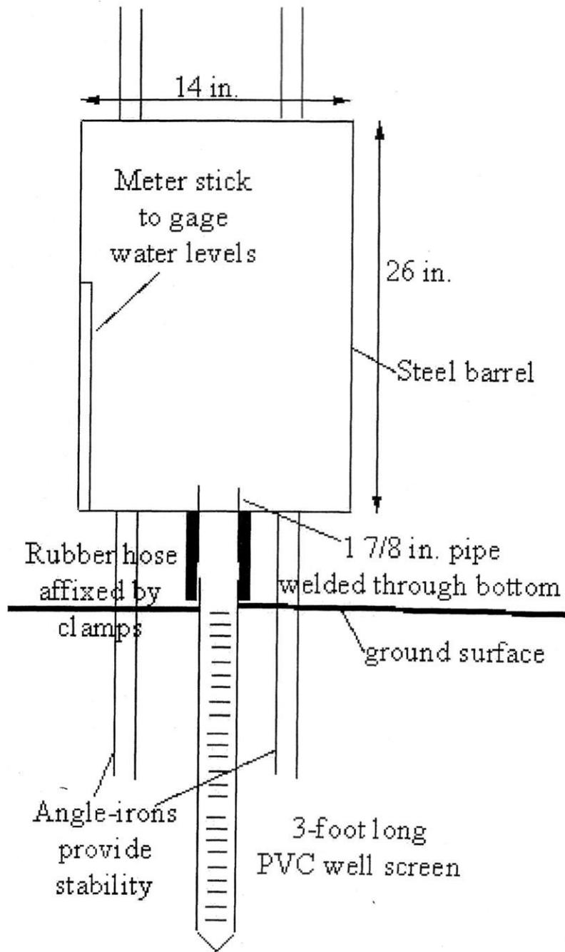
Figure 6. Water infiltration system diagram
