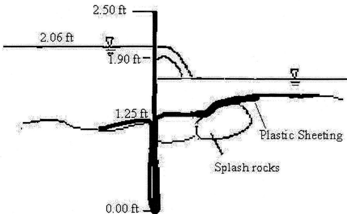
Figure 40. Channel profile at Syene Road weir, average flow conditions
