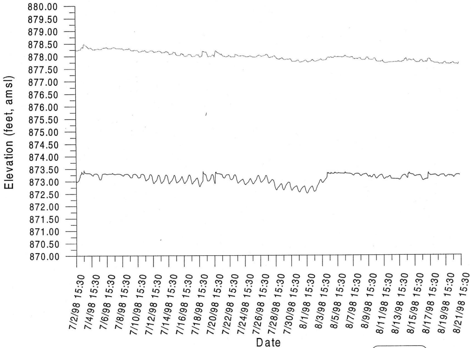
Continuous hydraulic head measurements,
