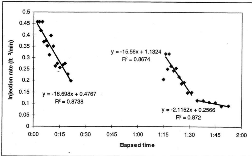
Figure 8. Water infiltration rate during well test
