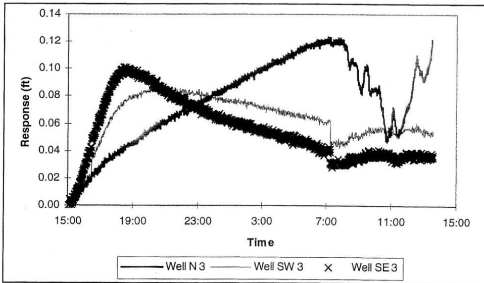
Figure 9b. Water levels in wells three meters from source
