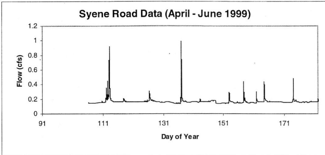
**Figure 45. Flows observed at Syene Road weir**
