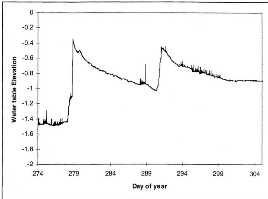
**Figure 14. Water table recovery from two October storm events at Syene Road experimental site**
