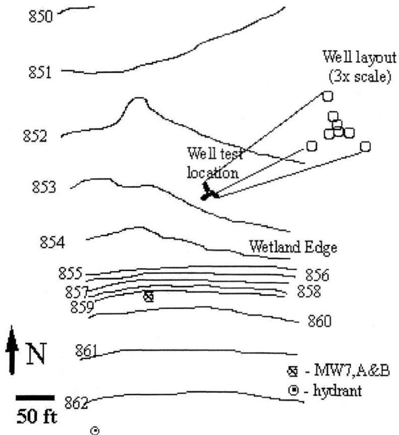
Figure 5. Well test layout
