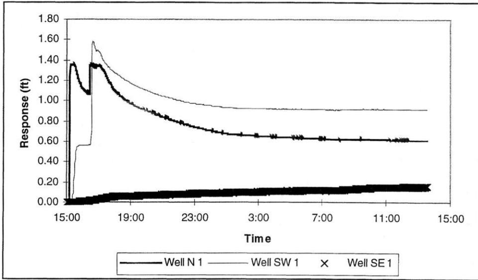
Figure 9a. Water levels in wells one meter from source
