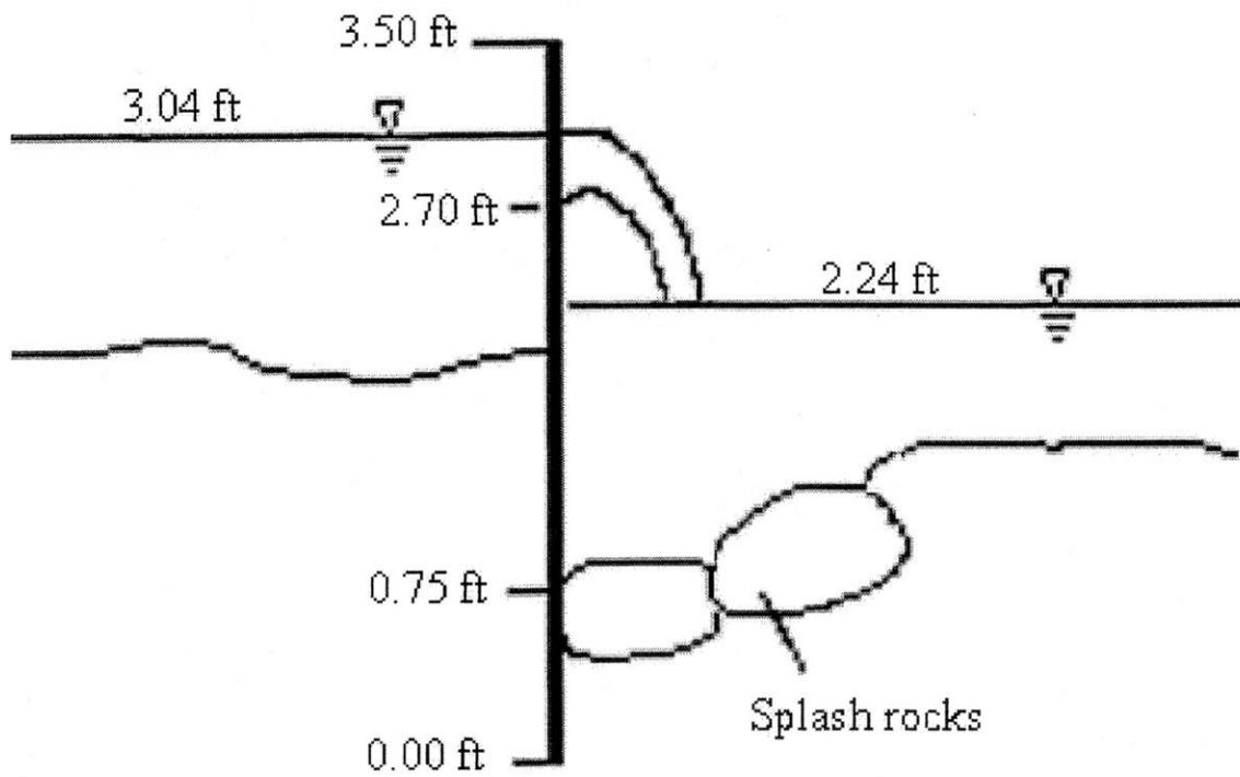
Figure 33. Channel profile at Gunflint Trail weir, average flow conditions
