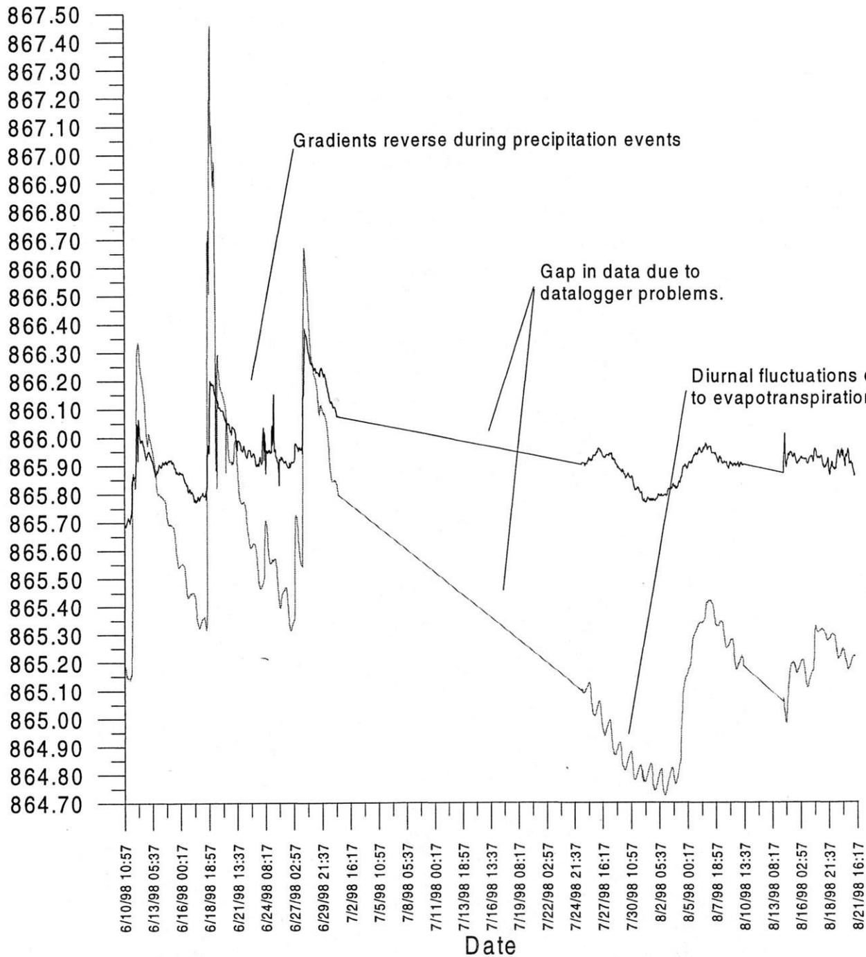
Continuous hydraulic head measurements,
