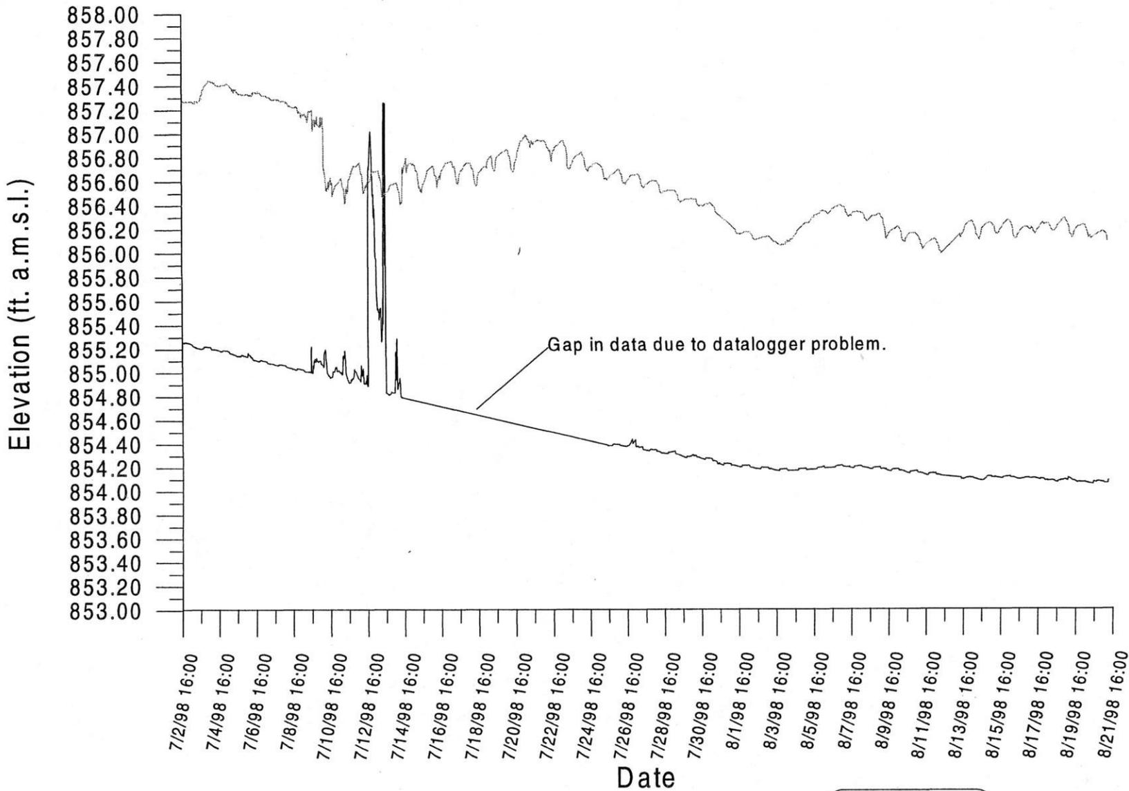
**Continuous hydraulic head measurements,
