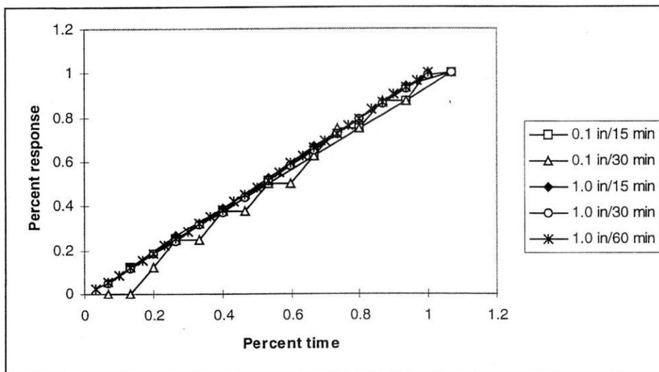
Figure 37. Relative gage response to simulated rainfall (two-minute intervals)
