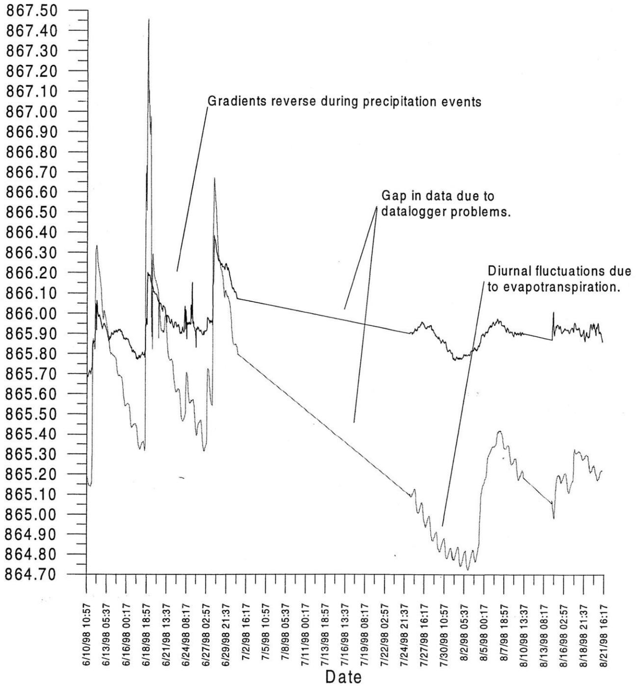
Figure 25. Continuous hydraulic head measurements at MW3A and MW3B
