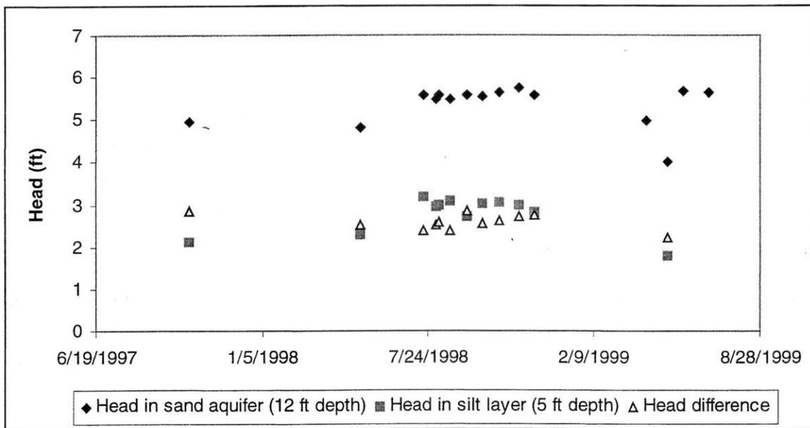
Figure 44. Hydraulic head measurements beneath Big Spring
