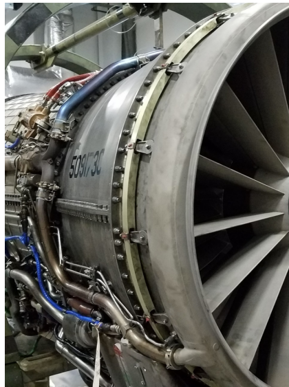
Figure 1.1: Turbine engine, consisting of different components fastened together using numerous bolts
