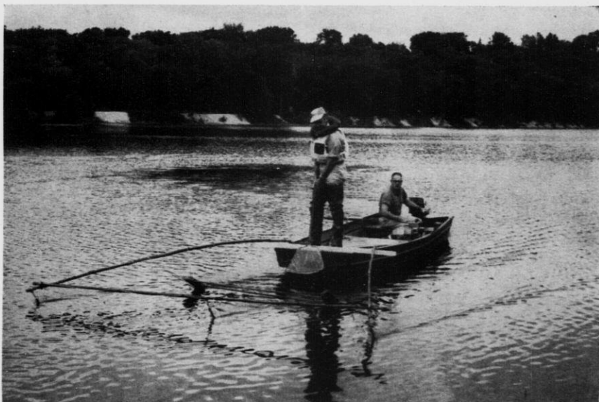
The "boom shocker" is a valuable new tool in sampling fish populations for research and inventory purposes.
