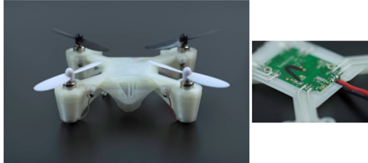
Figure 1.6: FDM printed functional quadcopter. Printed via Voxel8 with embedded electronics and endures structural loading [1].
