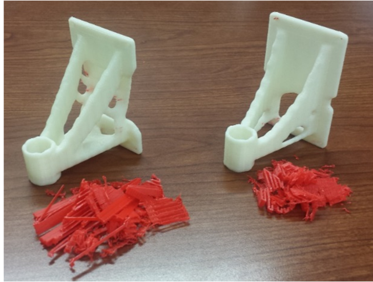
Figure 2.26: Printed mount bracket and the required support structures at 0.7 volume fraction.
