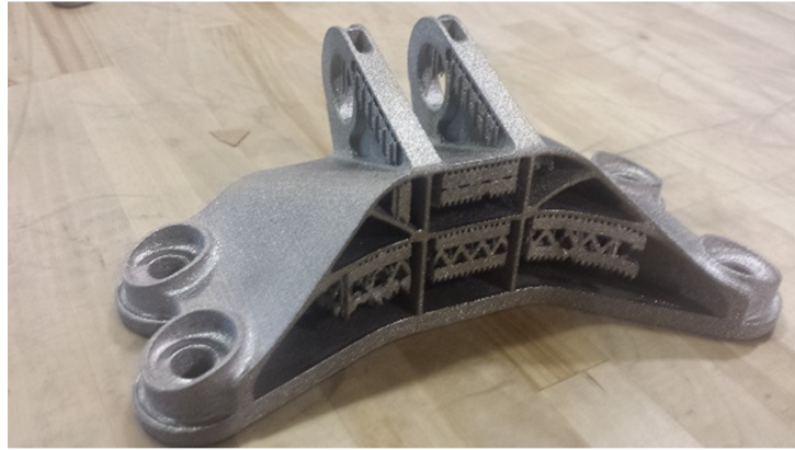
Figure 2.3: Optimized GE engine bracket printed by Arcam (EBAM) metal 3D printer.
