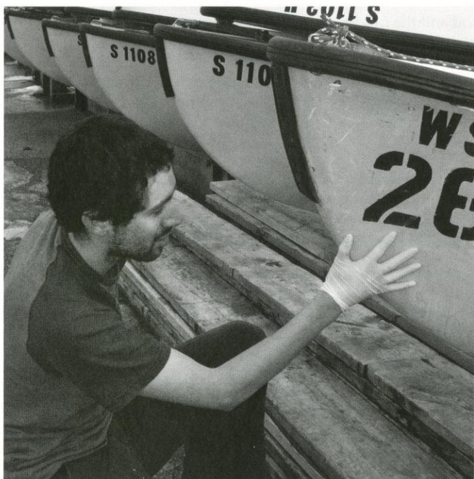
Photo by Jamie Tabaka: Rodolfo Perez examines the hull of a Hoofers sailboat for signs of biofouling.
