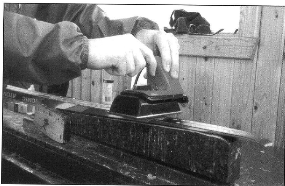
The wax is spread out evenly over the entire length of the ski with an iron.
