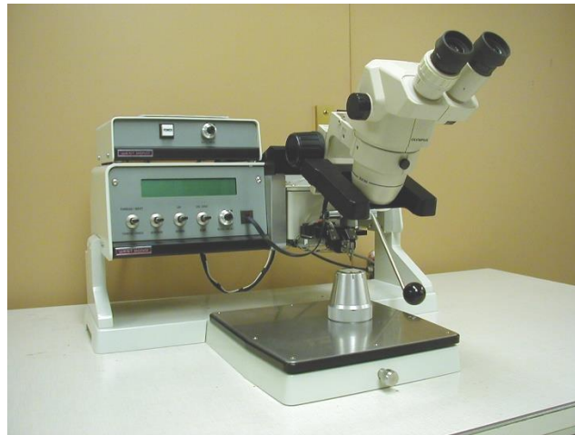
Fig. 5-12 Westbond 747677 Aluminum wedge bonder
