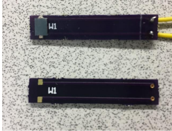
Fig. 7-4 PCB connection board for initial measurement
