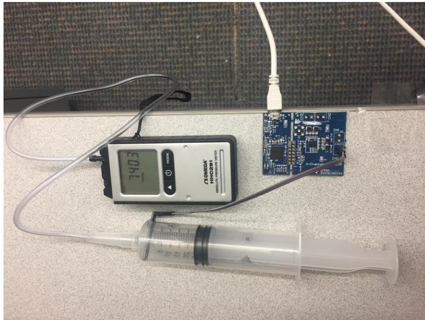
Fig. 7-8 Springe with piston, pressure sensor, digital pressure meter HHC 281 and sensor electronics FDC2214EVM
