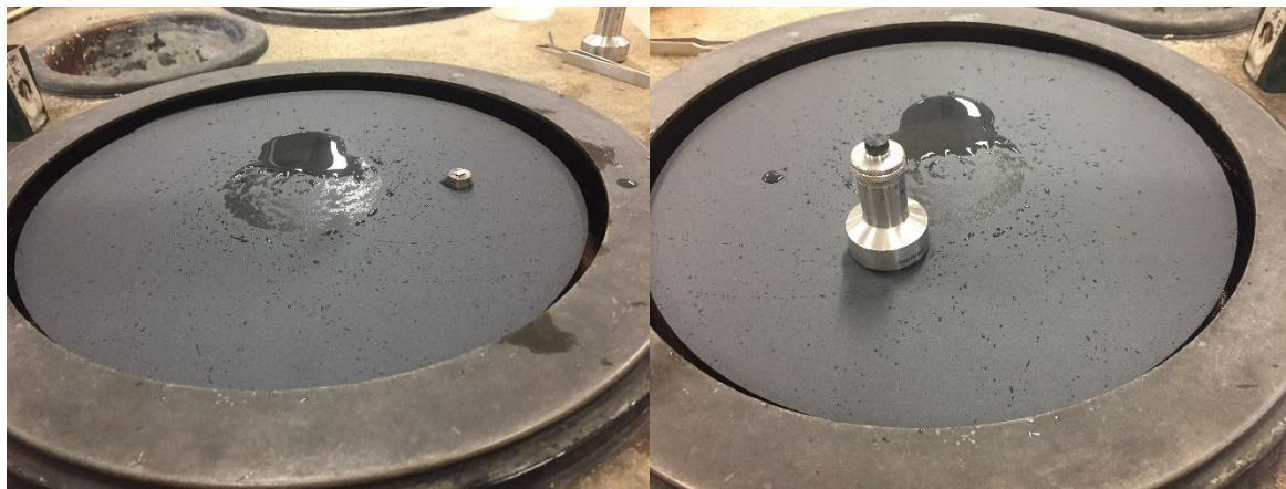
Fig. 9-20 (a) Sensor sample mounted on the tool for grinding (b) Grinding tool overview
