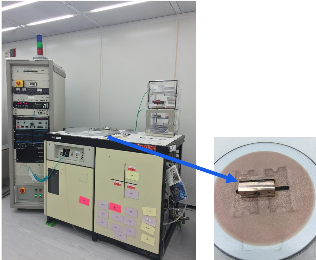
Fig. 5-11 (a) CVC sputter machine (b) Special holder put in chamber to fix the samples and expose sidewall
