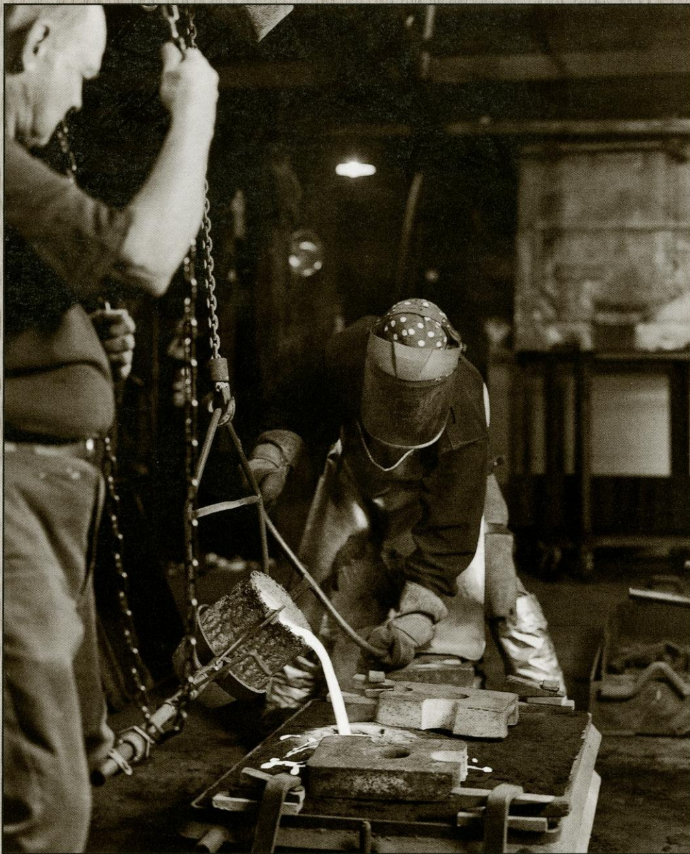
HOT METAL: Tom Pankratz pours molten bronze to make the 'Rededicated 1998' plaques.
