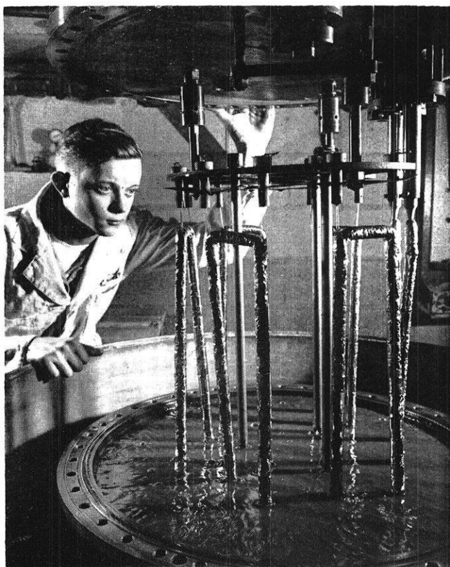
—Courtesy Westinghouse Engineer Zirconium bars in the process of formation.
