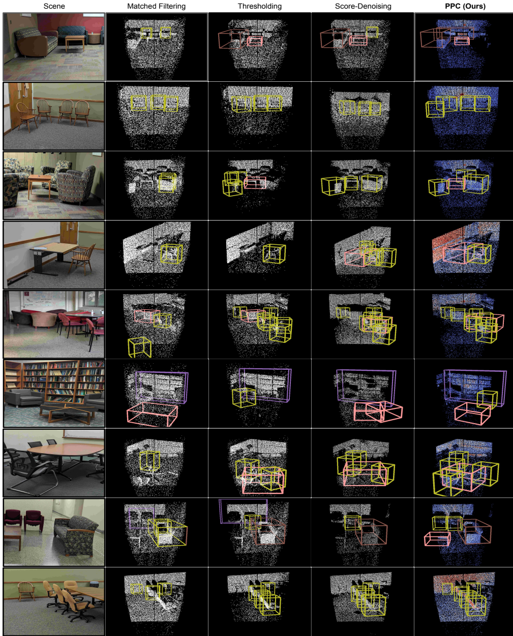
Figure 3.14: 3D Detection Results on Real Indoor Captures: Figure compares our method with the baselines under challenging low SBR conditions. Baselines fail to detect many small and farther objects, e.g chairs in the back of many scenes. PPC detects most objects ( e.g chair , table , and couch ) with tight bounding boxes.
