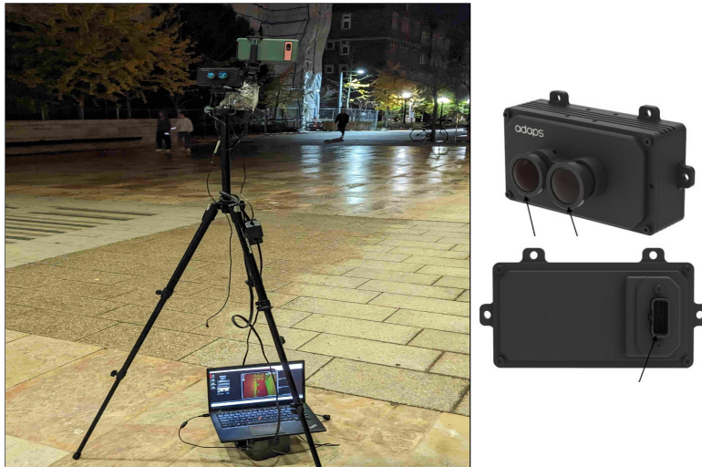
Figure 3.13: Outdoor Camera Setup: The Figure shows the front view of our Adaps camera setup (left) and the sensor (right).
