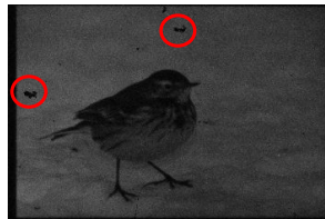
Figure 4.18: Artifacts in Real Captures from SwissSPAD2 camera
