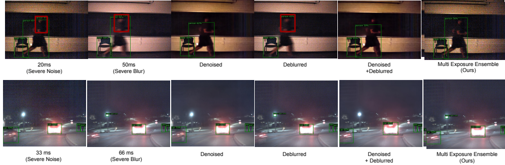
Figure 5.9: Object Detection Results on Real Captures: Scene in the first row contains an indoor scenario with two objects: a person (moving) and a chair (stationary). Single Exposures are severely affected by noise and/or blur: detect false positives or inaccurate bounding boxes. Scene in the second row contains a driving scenario with a car (moving) on the left and a traffic light (stationary) in the front. Single Exposures fail to detect the moving car or the stationary traffic light. The Multi-Exposure Ensemble approach (right) leverages multiple exposures and detects all objects with correct labels and tight bounding boxes in both scenes.
