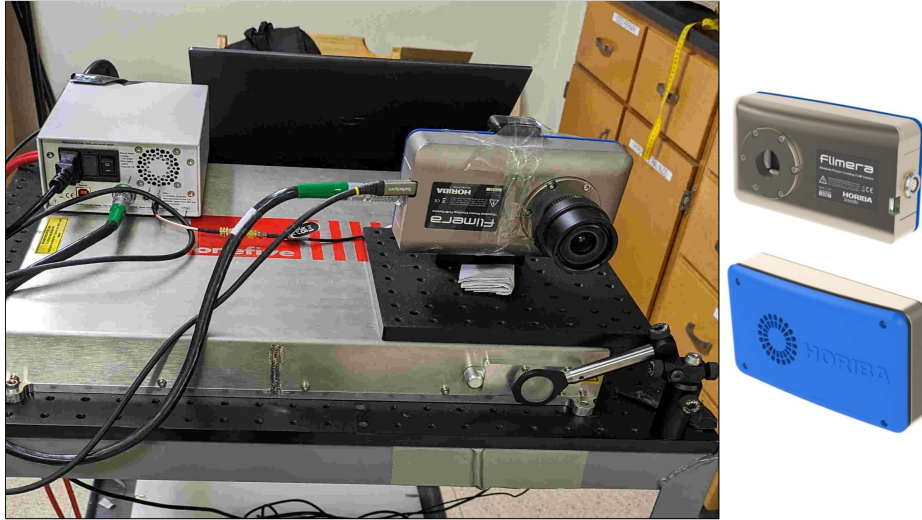
Figure 3.12: Indoor Camera Setup: The Figure shows the front view of our FLIMera camera setup (left) and the sensor (right).
