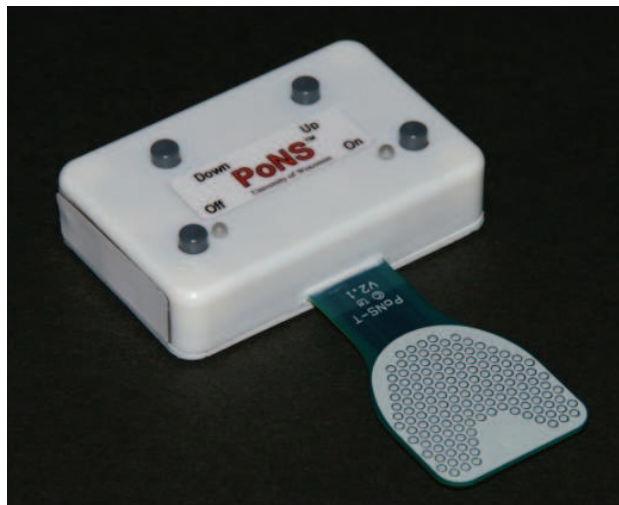
Figure 1.1: Portable Neuromodulation Stimulator used to deliver Cranial Nerve Non-Invasive Neuromodulation
