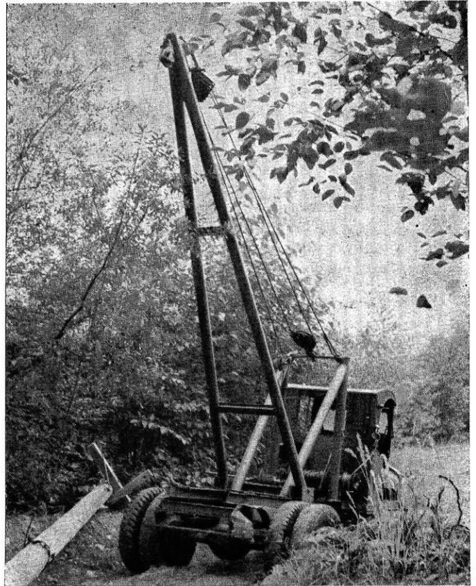
The Logger's Dream, a Truck Mounted Jammer —Courtesy U. S. Forest Products Lab., Madison
