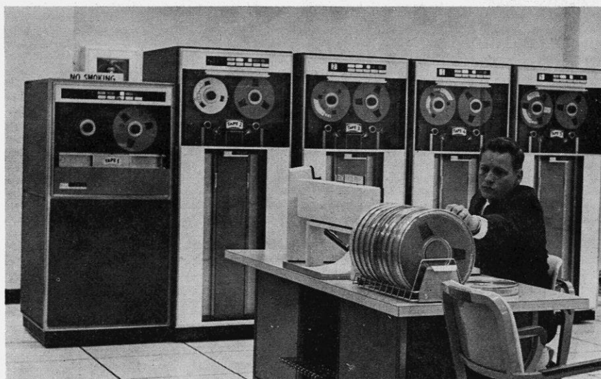
All new student records are being put on IBM tape and will be processed by one of the University's computers located in the basement of the new Administration Building. The picture shows the control console and the bank of tape processing computers which are used in handling the records of students now on campus.
