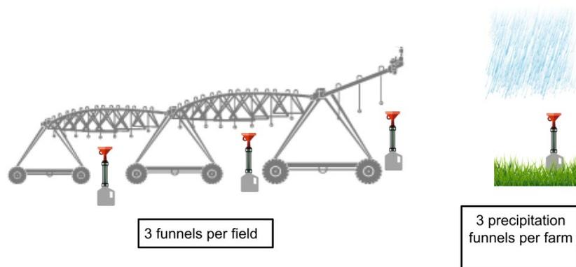
Figure S1. Passive funnel system used to collect irrigation water from a center pivot irrigation system in conjunction with rainfall measurements.
