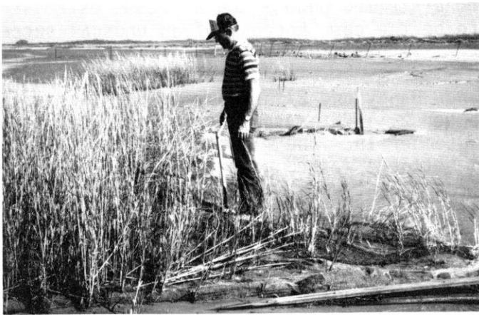
Figure 12. Smooth cordgrass in fabric mat at Bolivar Peninsula 15 months after planting.
