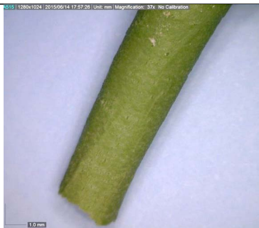
Figure 4.25d K0118 impression showing heavy wear and scratches inside the drill hole
