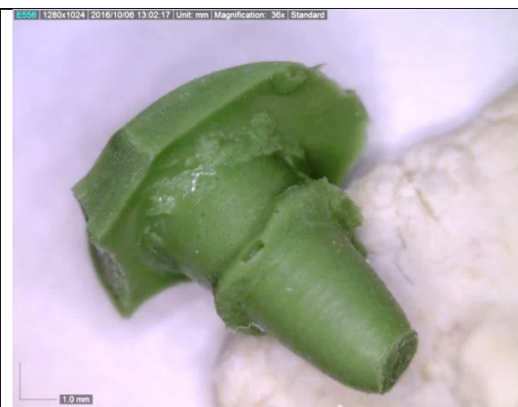
Figure 4.65 J0074 a visible flaw inside the impression
