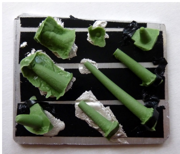
Figure 2.7 SEM samples mounted and ready for coating.*not to scale
