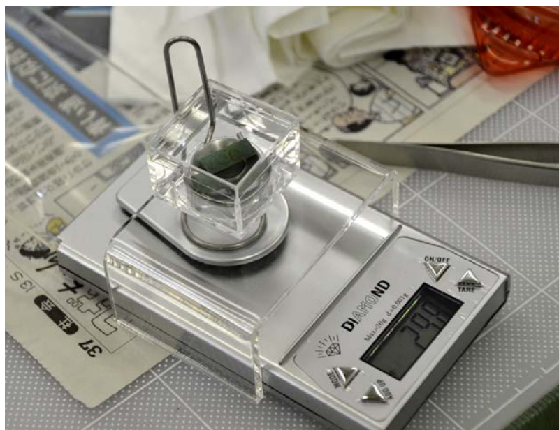
Figure 2.6 My specific gravity scale taking the water weight of a cylindrical jasper bead.
