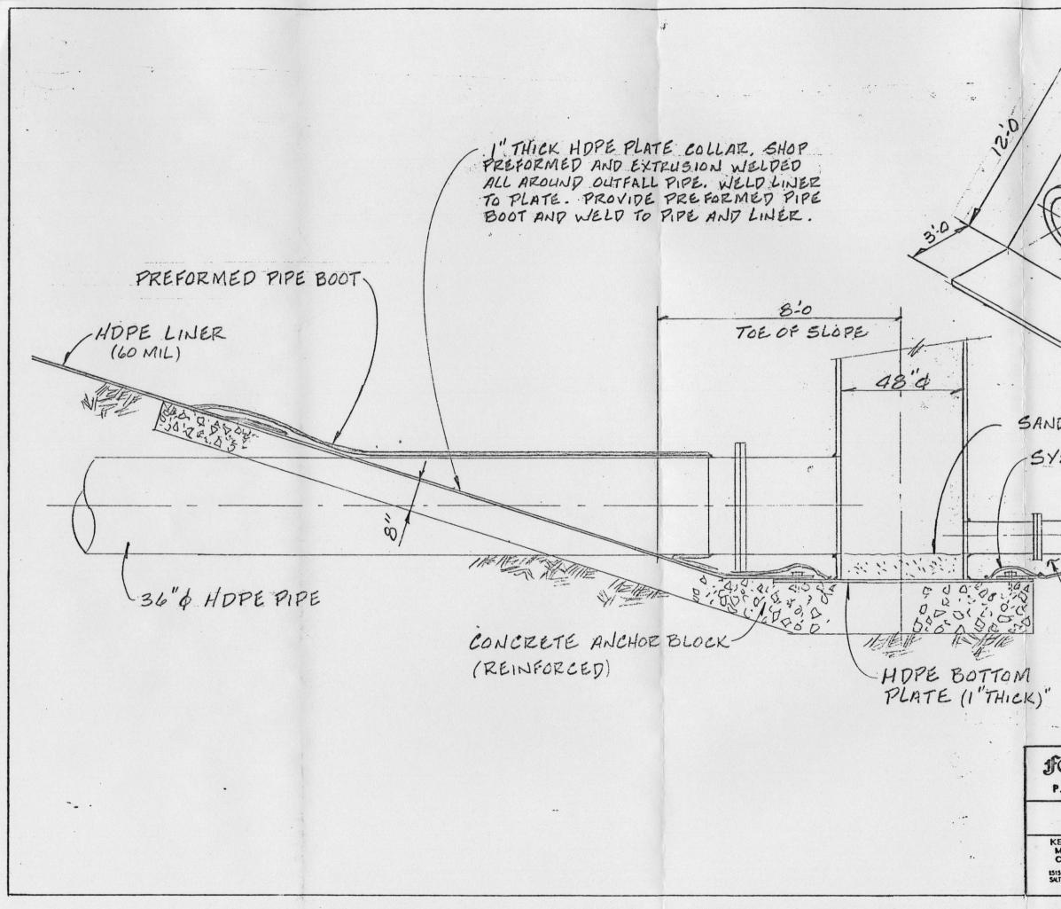
ISOMETRIC VIEW OF PIPE & COLLAR SAND CUSHION SYSTEM C ANCHOR 616 HOPE LINER BACKFILL PIPE HAUNCHES WITH IMPERVIOUS MATERIAL (TYP) JFORD, Bacon & Pavis Utah, Inc. ENGINEERS - CONSTRUCTORS P.O. BOX 58889 - SALT LAKE CITY, UTAH 84158-6809 BAD. DATE 11-89 FLAMBEAU PROJECT GLT SKETCH NO. LADYSMITH, WISCONSIN KENNECOTT MINERALS COMPANY B FIGURE NO 4-52 YPE II STOCKPILE DUTLET STRUCTURE 1515 WINERAL SQUARE SALT LAKE CITY, UTAH 84112 PIPE PENETRATION DETAILS SCALE NONE
