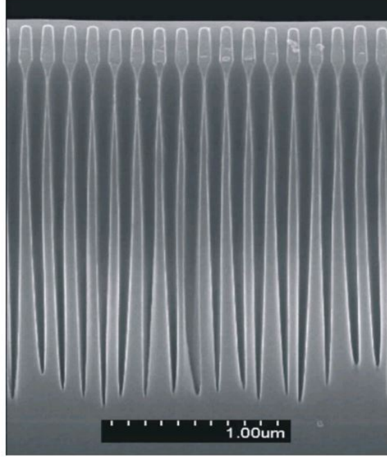
Figure 1.6: Incident auxiliary high-energy electrons to improve etching profile by neutralizing positive charge on sidewalls [39].
