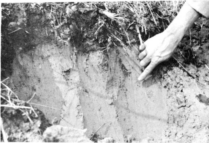
A wet mineral soil. The hand points toward mottles.
