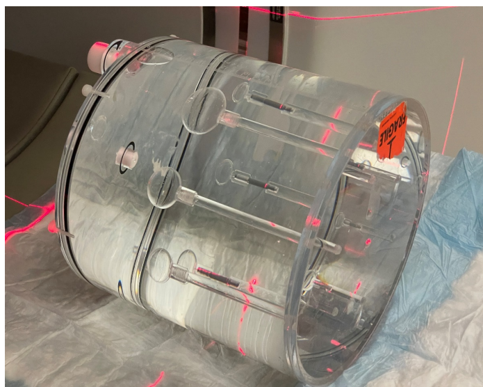
Figure 6: Jaszczak Flangeless Deluxe PET and SPECT phantom with a set of 6 hollow spheres.
