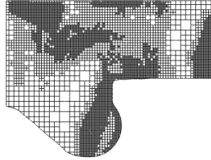
Figure 3.8: Representative GM 1.9L Converge simulation sector mesh at 50 deg. ATDC
