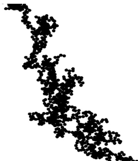
Figure 2.13: Space-fill representation silhouette of a soot particle with 1024 primary particles, a primary particle diameter of 11 nm, a radius of gyration of 22.5nm, and a fractal dimension of 1.76
