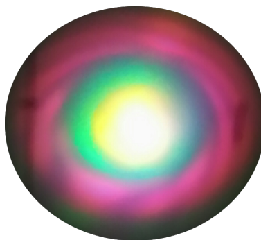
Figure J.1: White light generated in a \text{CaF}_2 window from 800 nm, 35 fs light. Photo taken in the Wright lab by Justin Earley.
