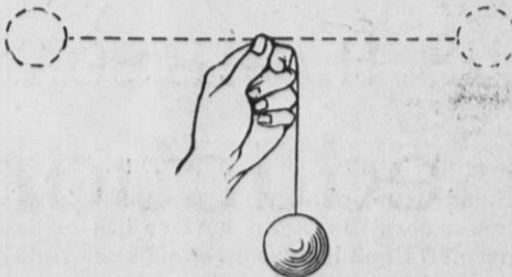
Fig. 5.—Diagram Illustrating the Running Balance—force, and it is only by adjustment of these two antagonistic forces that the face of a millstone can be maintained in a true horizontal position while running.
