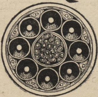
In the old days, it would have taken a pole line over 700 feet high to carry all the conversations that can go through a 2 1/2-inch coaxial cable.
