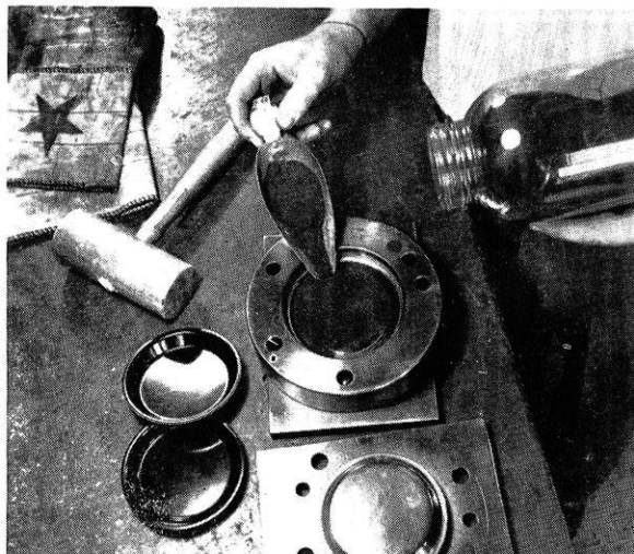
A variety of molded shapes can be made from the Forest Products Laboratories' waste-lignin molding powder.
