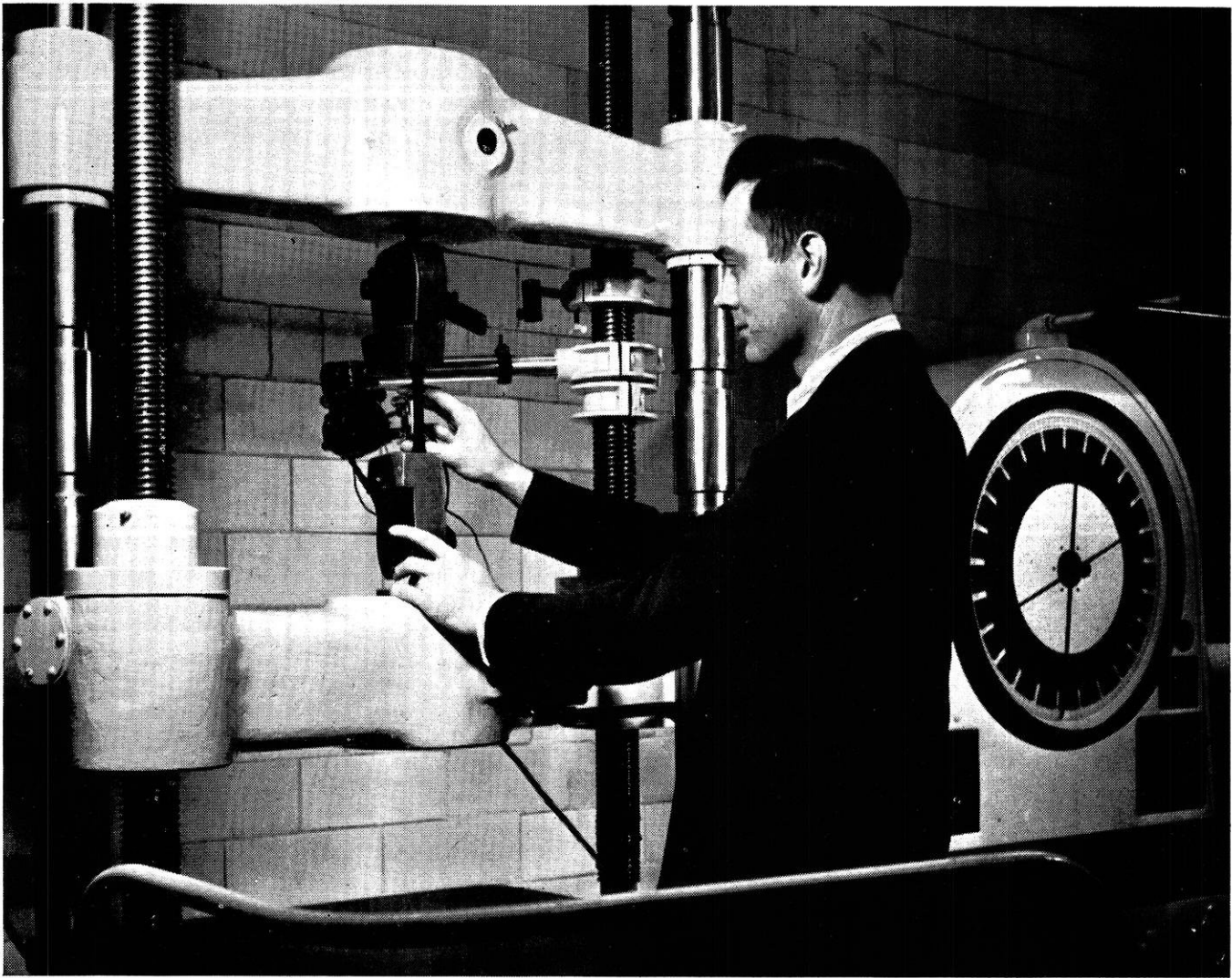
Working in a Dow physical research laboratory, this young man is operating a machine to test plastic materials.
