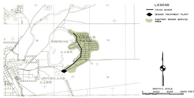
A second alternative sanitary sewerage plan considered for Browns Lake would provide sewerage service to only those residential areas located along the east side of the lake, with the residences on the west side of the lake to be eventually removed in order to provide restored "natural" lakeshore area. This alternative would also utilize a sewage treatment plant discharging to Hoosier Creek.
