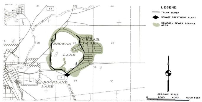
About 60 percent of the annual phosphorus contribution to Browns Lake is attributed to septic tank effluent seepage, seepage which also contributes to the high coliform bacteria counts in the lake. One of the alternative sanitary sewerage systems considered to eliminate these two forms of pollution would have a sewage treatment plant discharging to Hoosier Creek, with tributary sewers serving all of the lake community. Source: Harza Engineering Company and SEWRPC.
