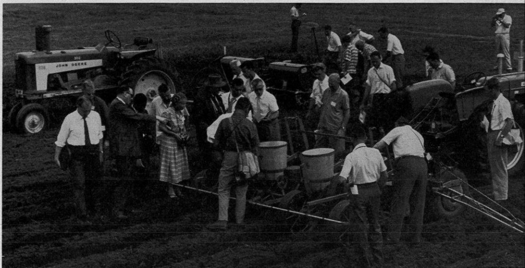
A demonstration of this minimum tillage wheel-track corn planter was one of the highlights of a field trip to the University's new Arlington farm. The revolutionary new corn planting method is being developed at the UW.
