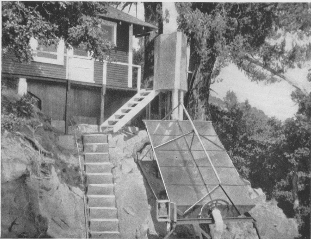
Abbot's solar cooker. Rays caught by the great mirror heat oil in the focus tube. The oil, circulating, bathes the cooking ovens in the reservoir above. The ovens stay heated night as well as day, and bake bread, meat, etc.
