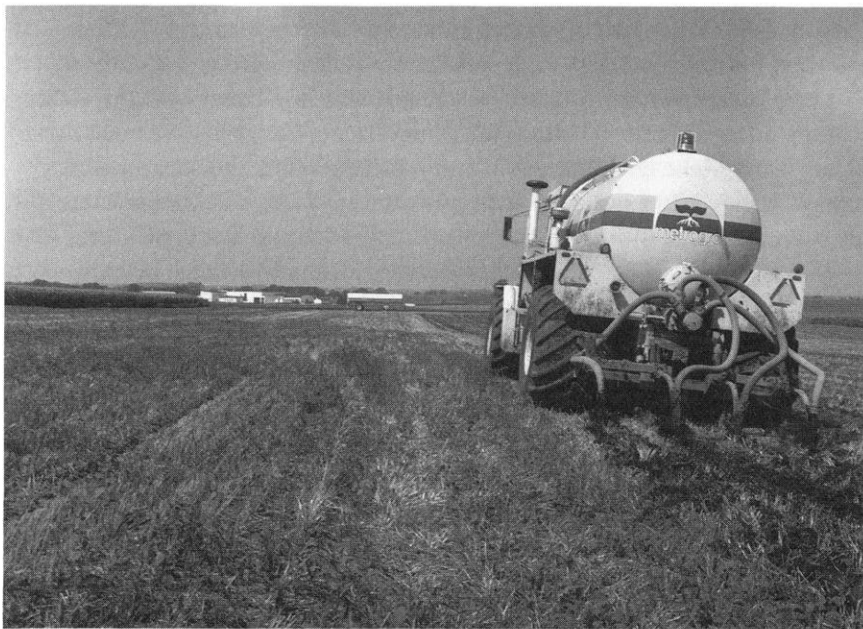
Injecting municipal sewage sludge on cropland. Departmental research has been crucial to effective and safe sludge applications. A.E. Peterson.
