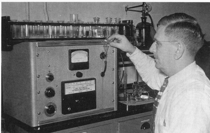
Walter Patzer making determination of available soil potassium using flame photometer. A.E. Peterson.
