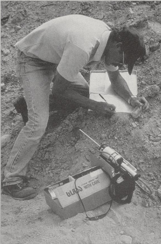
(left) It's tedious and costly to keep sampling soil around and under leaking tanks. Samples are analyzed to determine how wide an area is contaminated. Follow-up samples determine whether cleanup efforts are successful.
