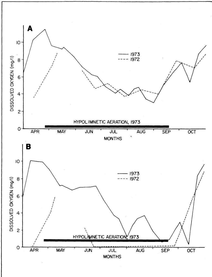
FIGURE 18. Weighted average dissolved oxygen concentration in Larson Lake, 1972 and 1973 (a) for the whole lake and (b) from a depth of 20 ft to the bottom.
