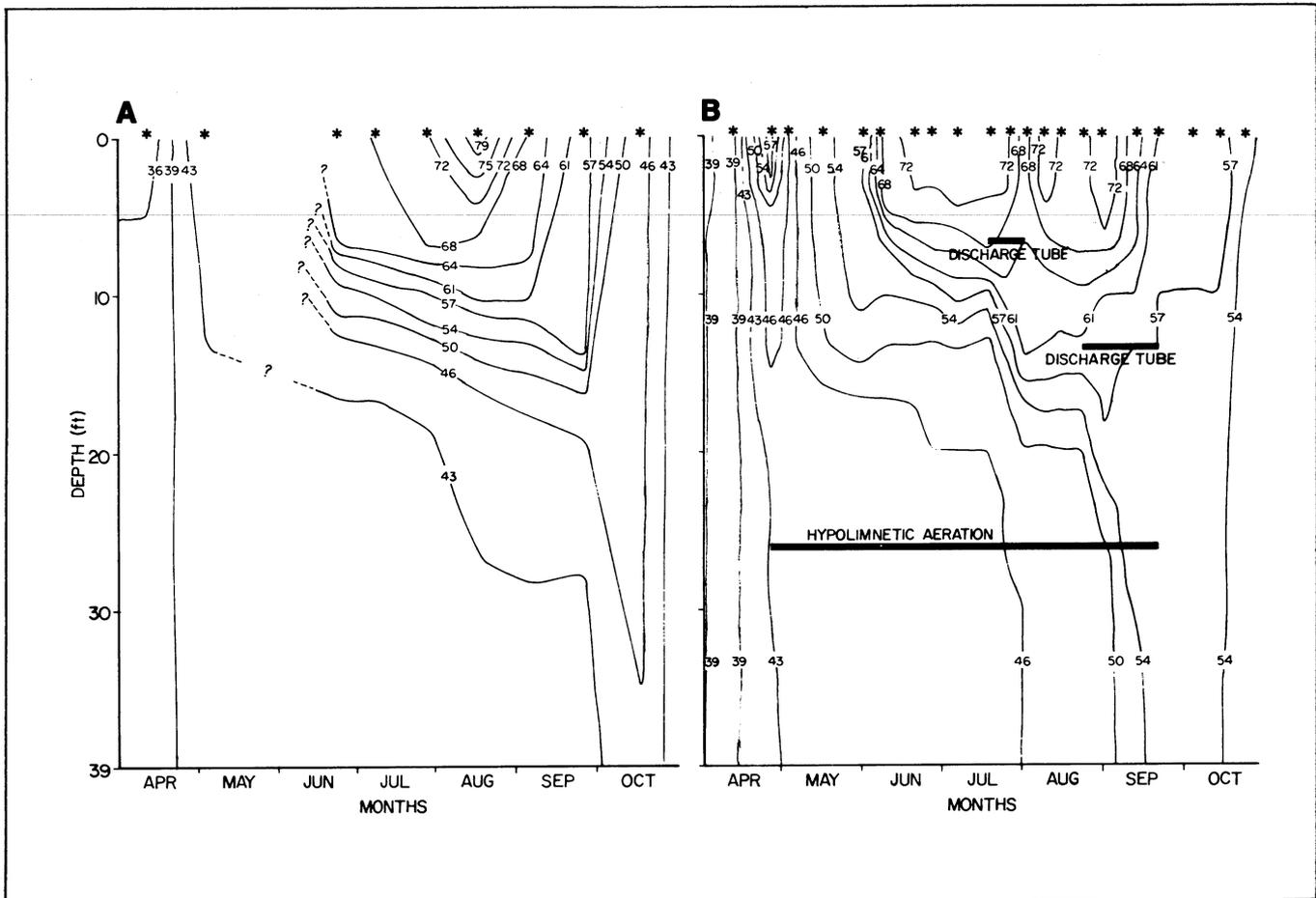
FIGURE 17. Larson Lake temperature isopleths (in° F) for (a) 1972 and (b) 1973. (Sampling dates are indicated by asterisks.)
