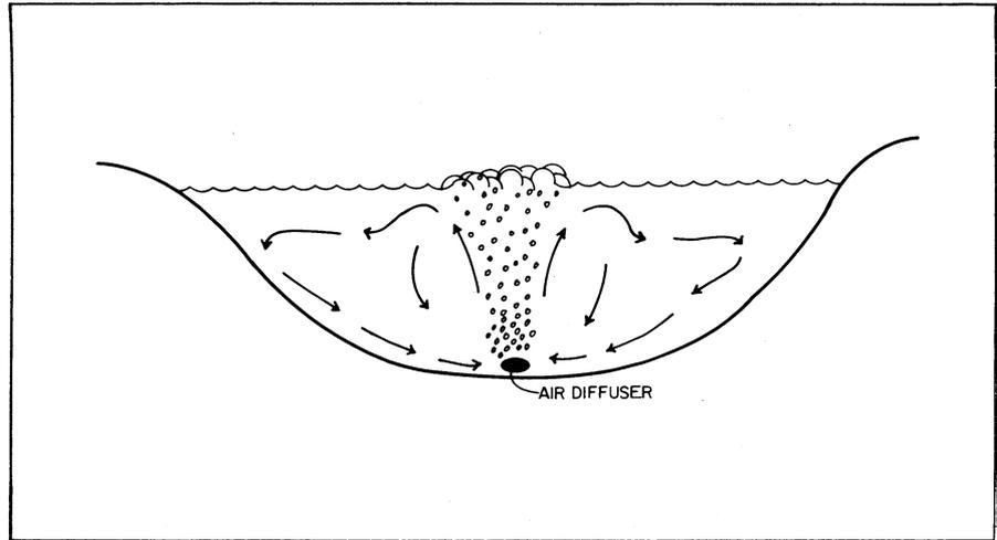
FIGURE 24. Diagram of water flow during lake destratification.
