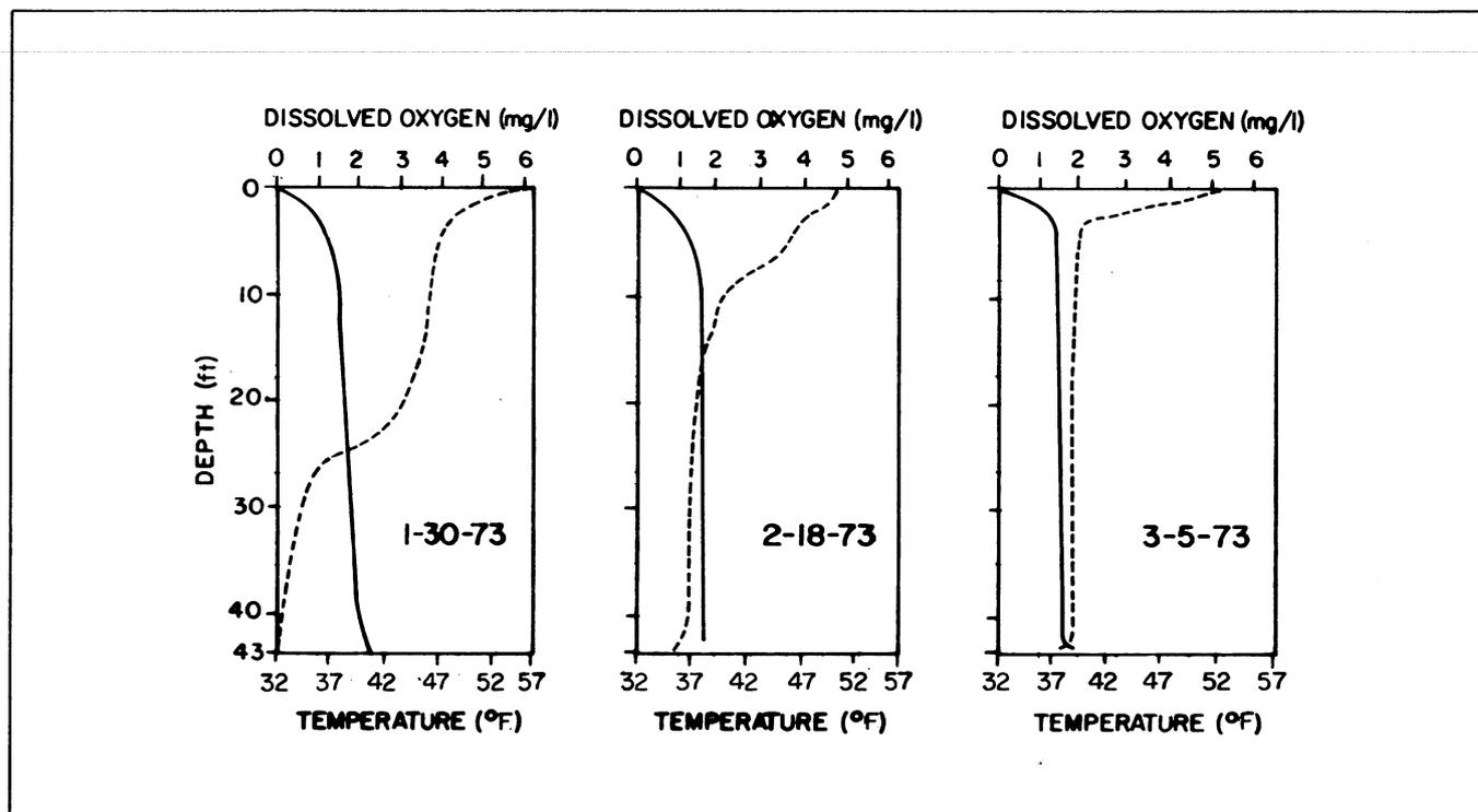
FIGURE 8. Dissolved oxygen and temperature profiles in Mirror Lake during winter aeration, 1973. (The aerator was in operation from 30 January to 8 March).
