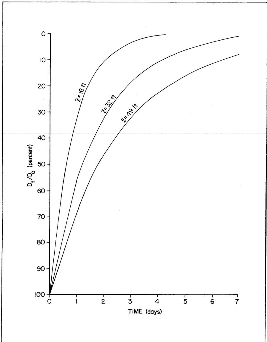
FIGURE 25. Natural (atmospheric) aeration of totally mixed lakes. ( $D$  is the initial dissolved oxygen deficit in mg/l,  $D_t$  is the dissolved oxygen deficit at time  $t$  in mg/l, and  $\bar{z}$  is the mean lake depth in m.)
