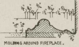
MOLDING AROUND FIREPLACE.
