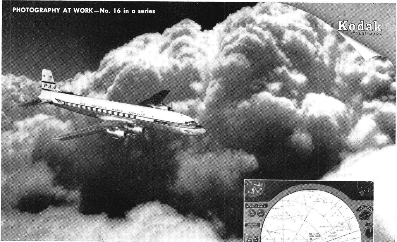
In the Arma Visual Computer, a single control selects the desired chart from as many as 700 photo slides. Each slide contains punched code holes which automatically tune in the corresponding Omni Bearing Distance station. The image of the plane is governed by a combination of the radio signals and the plane's gyro instruments.
