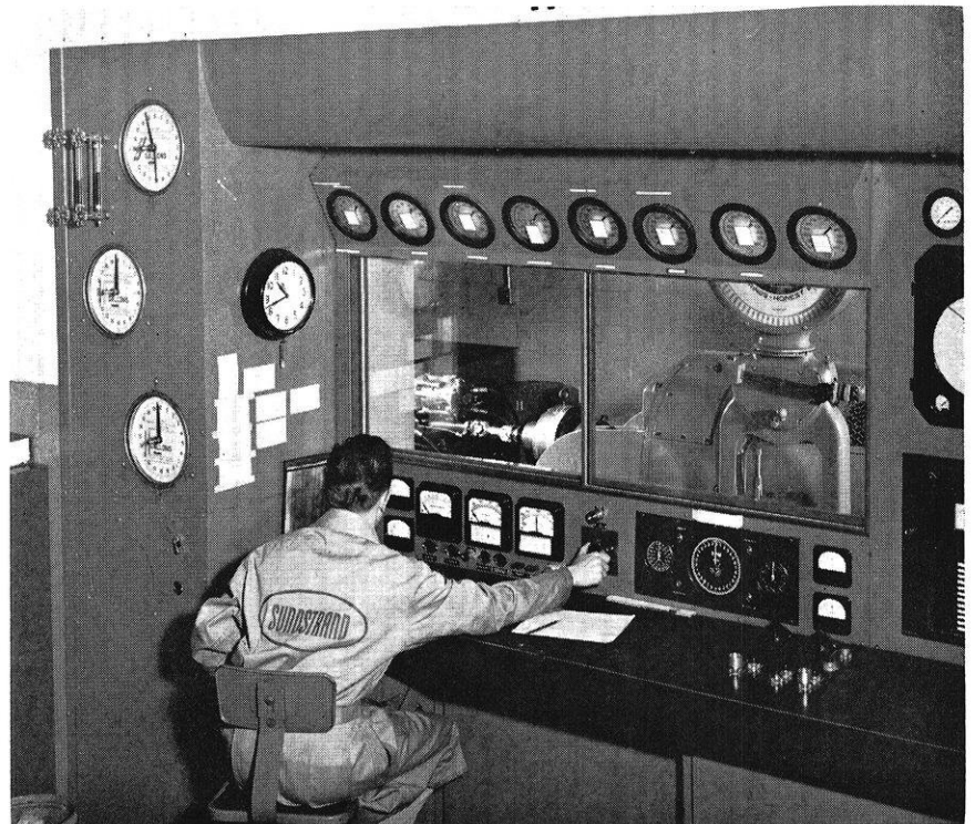
Typical test stand for product certification tests of equipment requiring a prime mover or absorption dynamometer.
