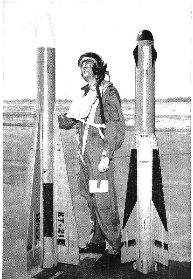
Falcon air-to-air guided missiles with both radar and infrared guidance systems are being developed and produced by Hughes engineers in Tucson, Arizona.
