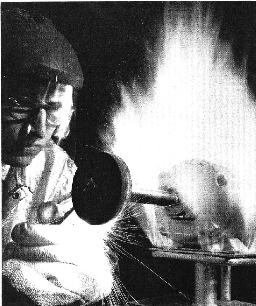
This motor is operating under severe temperatures of nearly 1000°F. over long periods of time and still give satisfactory performance.
