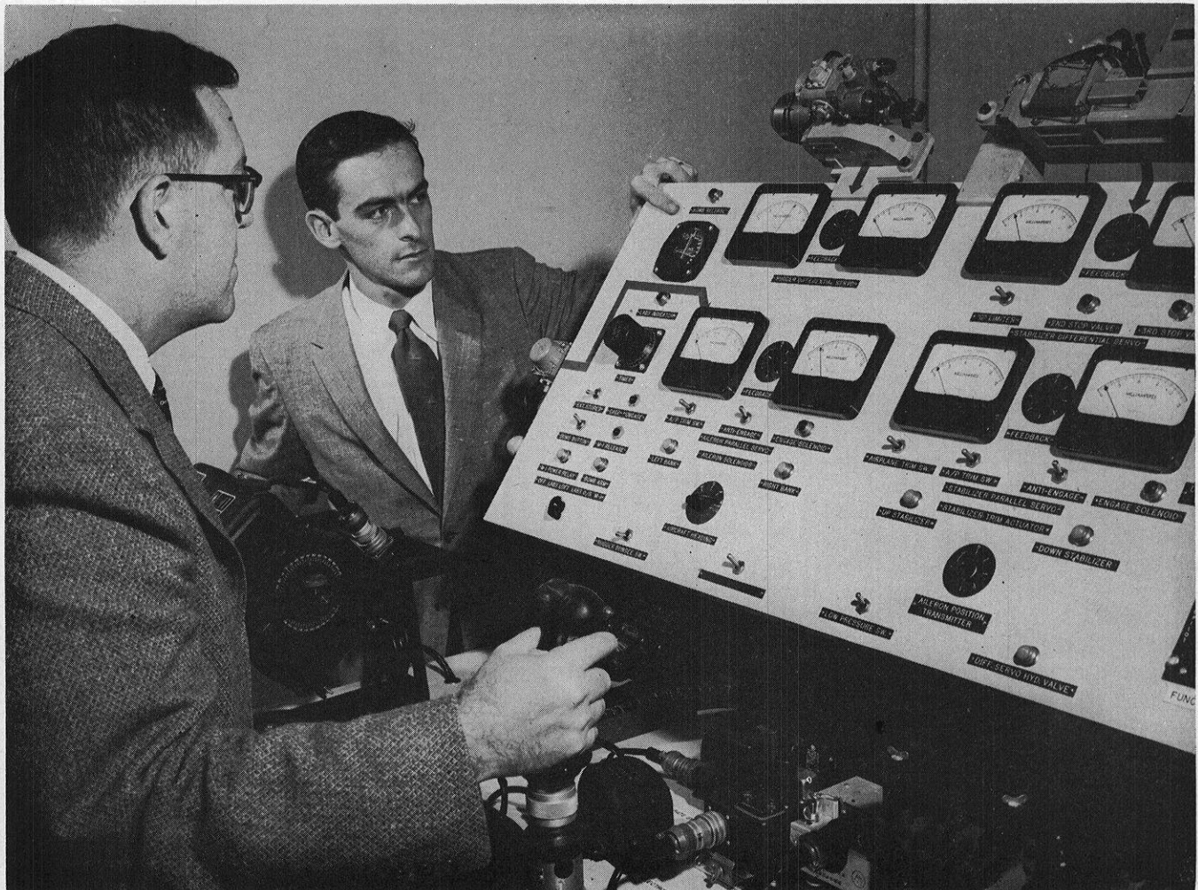
Simulator used to test auto-pilot equipment.
