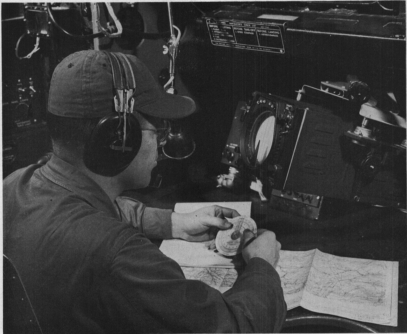
L to R, rear, are stabilizing gyro, and tranceiver units; front, radar screen and synchronizer unit, and master control panel for many different uses.
