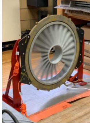
Figure 2.3-4 Integrated 7kW axial-flux SPM and propulsor-fan demonstration [71].
