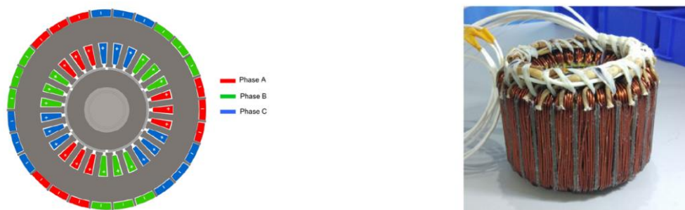
Figure 2.4-4 FT PMSM generator designed for internal turn-to-turn FT [119].
