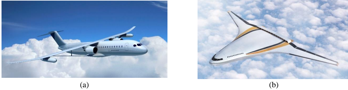
Figure 2.1-1 NASA N+3 Subsonic Fixed Wing Project aircraft concepts using electric machines: (a) Boeing SUGAR Volt; (b) NASA N3-X [59].
