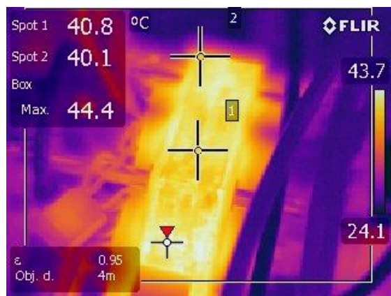
Figure 8.5-9 Thermal image of demonstrator stator after case 3 test.
