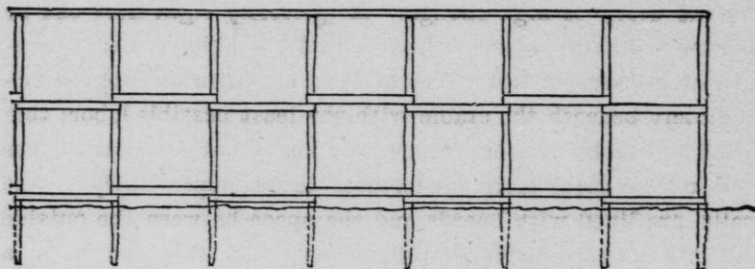
Side View of Frame, without roof rafters
