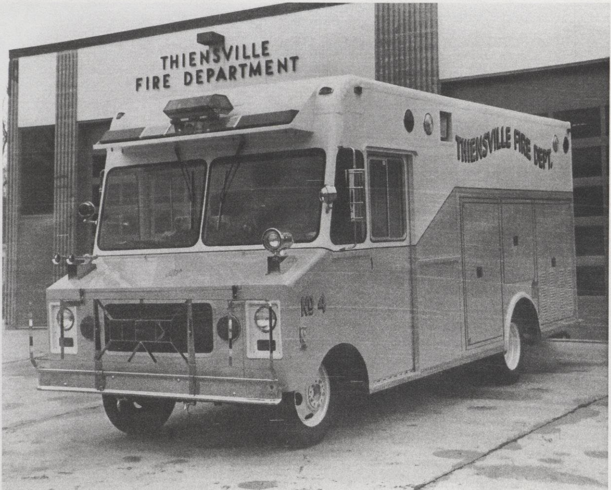
Service 554 – The 1982 GMC 3-D Apparatus equipment truck, carries additional fire fighting and EMS equipment.
