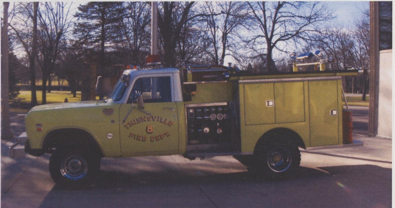
Engine 558 - The Internation/Pierce mini pumper used for brush fires and auto accidents, pumps 275 gallon per minute from a 250 gallon tank. Another accessory to the pumper is a class B foam proportioner.
