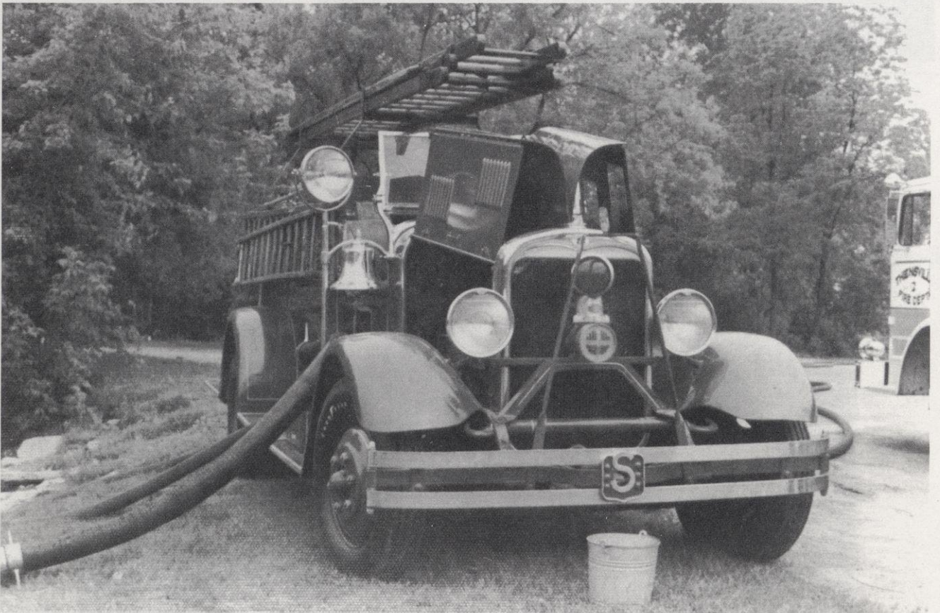
Even after being retired from active service, the department's 1935 Seagrave pumper was used in various roles, including supplying hose lines at training sessions. It is shown drafting from the Milwaukee River in 1973,
