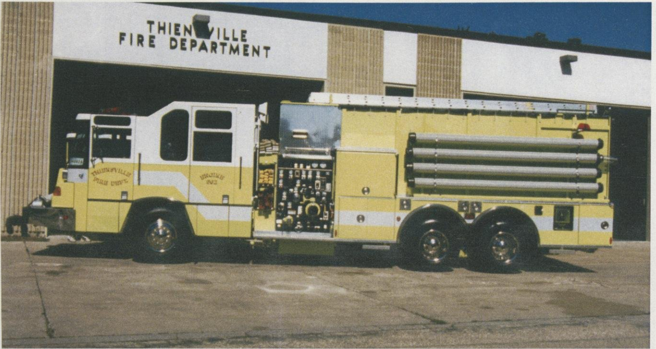
New 562 - 1997 Pierce Quantum tanker, 2000 GPM pump, 2000 gallon tank, class A foam system.
