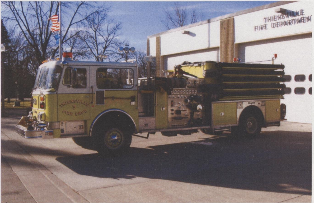
Engine 563, 1984 FWD pumper, 2000 gallon per minute pump from a 1000 gallon tank. It is also a mutual aid engine.
