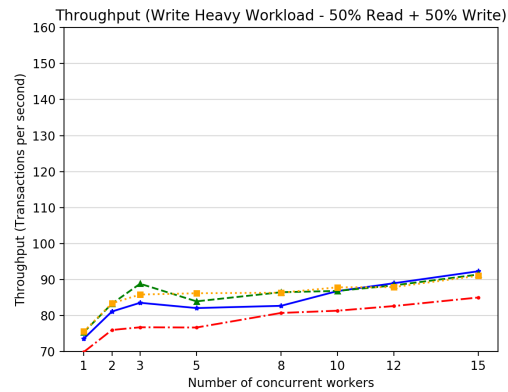
Figure 2.5: Transactional workload performance improvement due to Hustle, as compared between different write modes. This experiment altered the ratio of reads and writes in TATP, increasing the number of writes per read.
