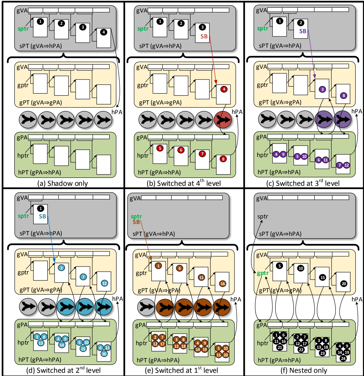
Figure 5.2: Different degrees of nesting with agile paging in increasing order of page walk latency. Starting point for each is marked bold and green.
