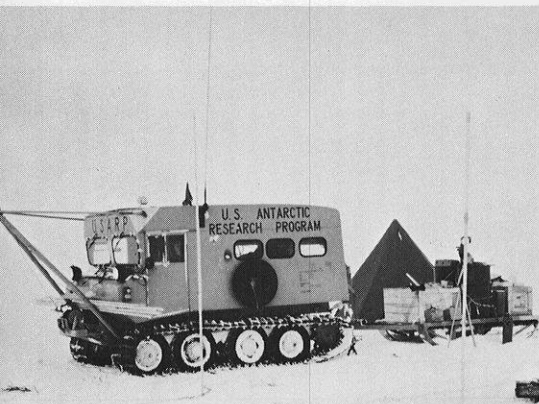
The Trackmaster, part of the specialized equipment developed for use in polar regions, carries personnel and light cargo on sleds.
