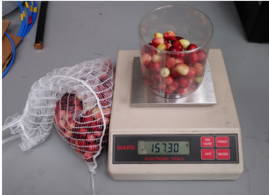
Figure 4.13: Setup for measuring the harvested cranberry yield with the MARS MS 200 precision scale.
