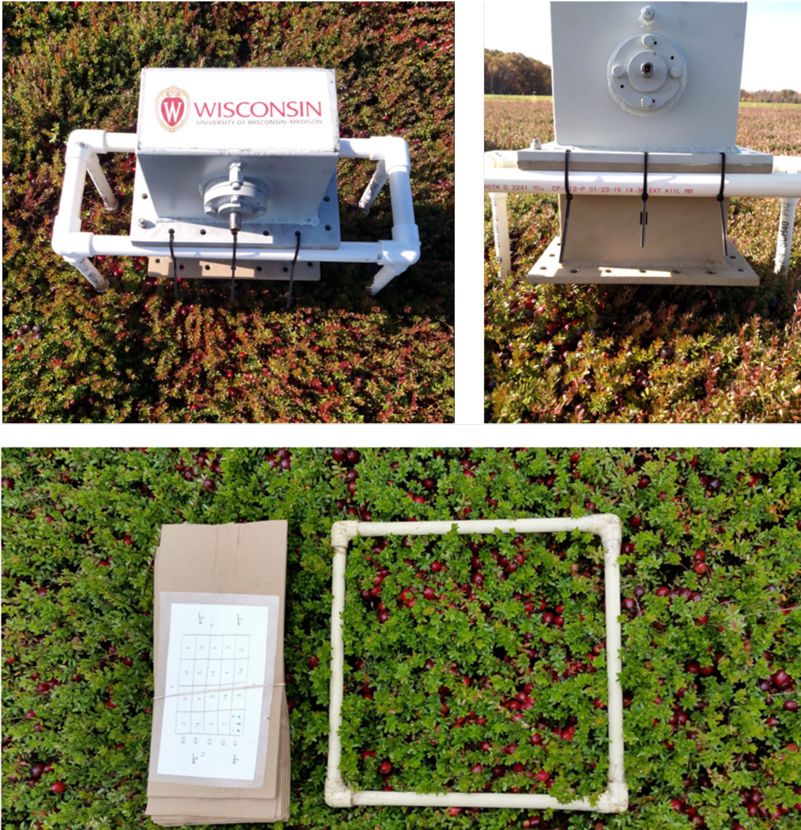
Figure 4.11: A rectangular open-ended waveguide (WR975) mounted above a cranberry canopy in central Wisconsin (top, right and left). A 1-ft 2 marker delineating a site for sampling the cranberry bed yield (bottom).
