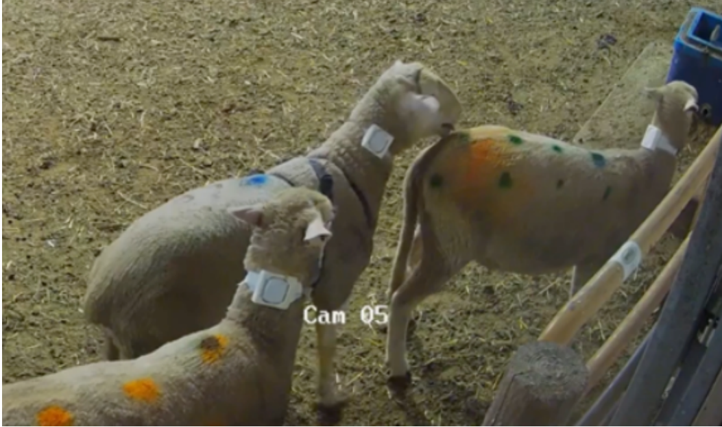
Figure 3.2 Still frame from video recording showing 2 ewes and 1 ram wearing custom collars affixed with the real-time location sensors in 3D-printed housings. The ram wore a black marking harness, and each ewe's back was painted with dots to allow identification from the video.
